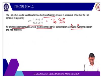
In the second one problem is the Hall effect can be used to determine the type of carriers present in the material. So Hall effect can be used to determine the type of carriers present in a material. Now so that Hall constants R is given by this equation. So Hall constant R can we measured from the other major quantities. So this is the expression for intrinsic semiconductor where n i is the intrinsic carrier concentration. m n, n p are the electron and hole.
