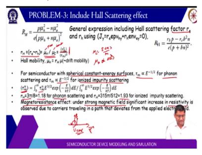
Now what is the significance of this scattering factor, electron and hole scattering factor? They are basically the ratio of mu h by mu c. So this is the hall mobility and this is the conduction mobility. So conduction mobility expression we use in conduction current. So J is equal to n e mu e. So they are the mu e is conduction mobility.
