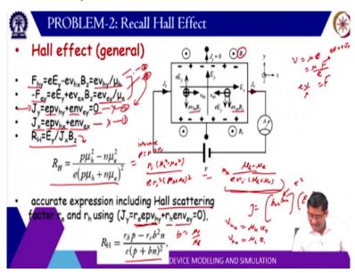
So now here if you see here, again the same scenario basically. The voltage is applied and in the x direction current is flowing and the magnetic field is in B z direction and both electron and holes they will experience force in - y direction due to q into v cross B. And then there is a value in net resultant electric field and this electric field will be in the opposite direction for the electrons and holes.
