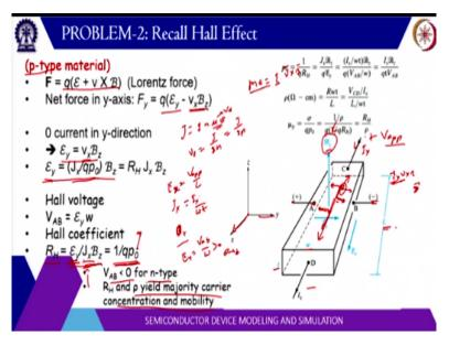
So consider a piece of semiconductor, a bar of semiconductor, where along the, this is the x axis, this is the y axis, this is the z axis. Along the x axis some potential is applied, let us say V applied and then current is flowing I x and the area of cross section we know this is w this is t and the length is some l. And there is a magnetic field in the z direction.
