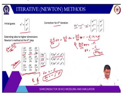
So let us say we start with initial guess. So zero is the initial guess. That is psi 0, n 0, p 0 are the initial values that we have assumed. Then for any arbitrary k-th iteration we can estimate omega k 1 s and difference of omega k plus 1 minus omega k will be delta omega k. And this is basically for the k-th step. This is the B prime right, the derivative. So we have del F by del psi, del F by del n, del F by del p.
