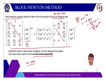
And that is called block iteration scheme. So here we have again created the same thing w is equal to M w. So you see here, this is taken, this diagonal matrix is taken. This is a lower triangular matrix. And then there is upper triangular matrix here with diagonal element zero. So if you see here they are exactly same equation. So what we have done, for these values, we have taken the previous iteration value.
