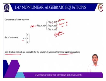
In this lecture, we will discuss the solution to nonlinear algebraic equations. Now let us consider a set of three equations. So as we have discussed, there is a Poisson equation, then there is a continuity equation for electron and continuity equation for holes. So these are the three equations. And if you notice, these three equations are not equation of one variable but they all involve the three variables.
