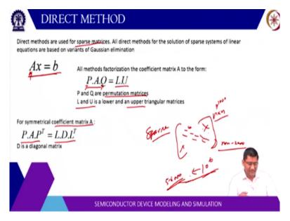
Then what we have discussed are the iterative methods. Other methods to solve the semiconductor equations are the direct method. So there we have this algebraic, now after the discretization we get algebraic equation of the form Ax = b. We can solve it iteratively or we can solve it directly. So what we do we again this convert A into upper triangular and lower triangular matrix.
