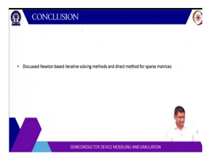
So in this lecture we have discussed Newton based iterative solving method and the direct method for sparse matrix. Okay. These techniques are used for this direct methods. They are used for sparse matrices. And sparse matrices are those where nonzero elements are actually very few, so diagonal and some nearby elements are nonzero. And most of other elements are actually zero.
