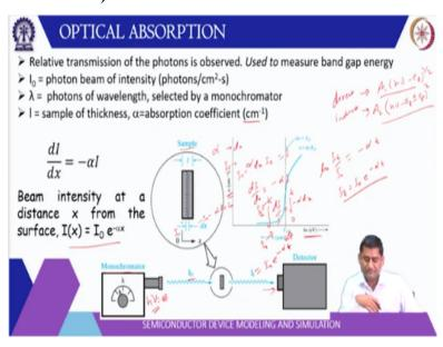
Now how do we measure these properties? So for example, using optical absorption, so we have this monochromator here. From this we select certain frequency. So e is equal to h nu will be the energy of this photon. And then we will sign it on a sample and see the transmission characteristic. So how much light is transmitted and that will also tell you how much light is absorbed.
