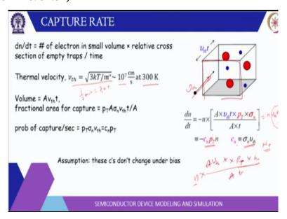
So this is the process basically you can see. Then let us write the capture rate, how these carriers are captured. So you can piece a, you can consider a piece of semiconductor here. Let us say we consider one area of cross section and this is the velocity of this carrier. So velocity can be assumed at room temperature is a thermal velocity. So half my square is equal to 3 by 2 k t.
