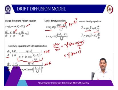
Now, let us recall the drift diffusion model, so, there is a charge density and the Poisson equation. So, generally, the poisson equation is written like this d 2 psi by dx square. So, here, psi of potential is equal to minus rho by epsilon times p - n + N D + - N A. Now, these are fixed charge, so, they can return as c. So, this is – rho by epsilon times p - n + some C. And n can be written as n i exponential q psi – phi by kT.
