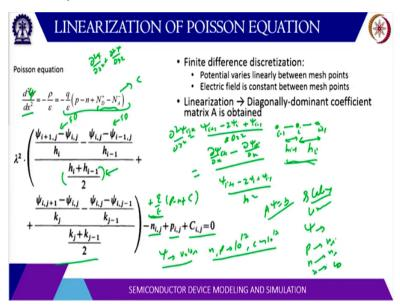
So, this we have already seen that d 2 psi by dx square is now, this is I have written for 1 dimension but for 2 dimension it will be d 2 psi by dx square + d 2 psi by dy square. Now, d 2 psi by dx square, we wrote that d 2 psi by dx square is psi at point i, K psi i + 1 - 2 psi i + psi i - 1 divided by 2 delta x square. Now, here it is shown for non uniform grid. So, this can also be written as d 2 psi by d axis.
