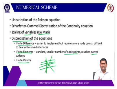
Now, numerical scheme so, once we scale and linearize then we use a discretization. So, for Poisson equation the discretization is normal finite difference, discretization and that is with respect to the potential. And scaling of the variable is attributed to De Mari a scientist introduce this technique. Then of course, this discretization that we have discussed, is at some level basically. Because there are different methods of discretizing it.
