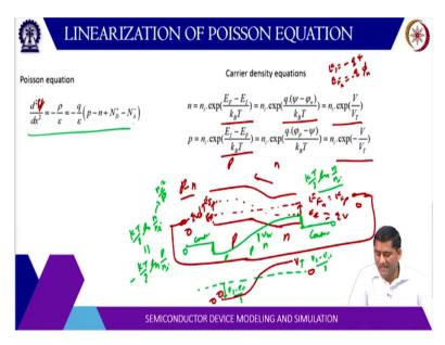
Now, linearization of the Poisson equation. So, this is d 2 psi by dx square is equal to minus rho by epsilon. So, this is -q by p - n + N D + - N A by this is the equation. And then the carrier density equation you have seen different forms E F - E I by kT then that is also written as q psi - phi n by kT where E = -q psi and E F = -q phi, so, n becomes phi N and p become phi p. So, this basically get reverse.
