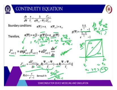
So, what you will have basically? you will have basically this is n i then this is n i + 1 e to the power psi – psi i by V T –1 e to the power psi i + 1 – psi i, i by V T – 1 and this is 1 – this thing, so, this will be denominator will be same as this 1 and e to the power psi i + 1 - i, i by V T – a to the power psi – psi i by V T. So, e to the power psi V T for n i + 1 coefficient is positive for n i the coefficient is negative that you can easily see here.
