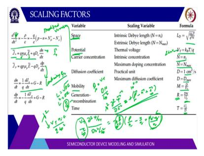
So, these are the different scaling things. Now, let us apply this to Poisson equation d 2 psi by dx square. So, here, if you write d 2 sin a dx square, so, d 2 psi. Now, psi we have to scale the potential is to scale with V T. So, what we can do? V can divide by V T and V can multiply by V T then dx square. Now, dx square, it will be divided by length and the length will be your space there is a debye length.
