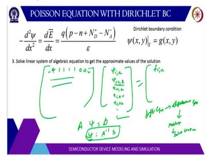
So now, what we do? We have this algebraic equation. Now, this algebraic equation can be written as in terms of matrix. So, these coefficients so, this coefficients can so, for example, psi i, k. What is the coefficient is 4 - 4 and then h square can be taken to other side, so, it becomes h square times f. So, what will happen here? If you write in terms of let us say psi of i, k psi of i - 1, k. So, psi i, k the coefficient is - 4 here i - 1, k. The coefficient is 1 here.
