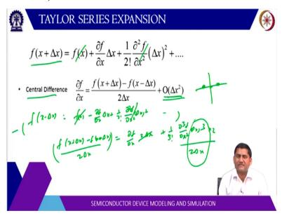
Similarly, for double derivative also, we can write so, double derivative so, let us try the central difference first. Now, central difference the advantage of central difference is that it is
