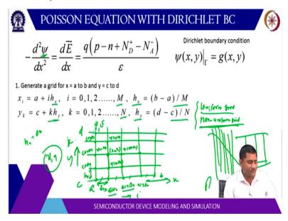
Now, how to solve the Poisson equation with Dirichlet boundary condition. So, the first step is basically is to create a grid. So, let us say this is your reason here. So, this is your x axis,
