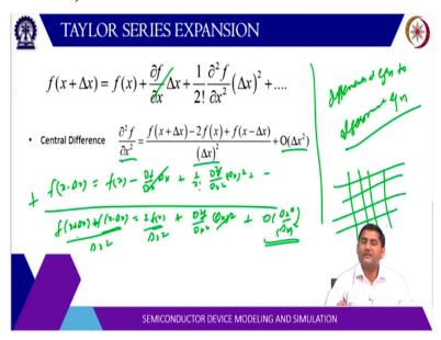
Similarly, for central difference f of x + delta x here we consider both side x + delta and x - delta x. So, let us write f of x + delta x because f of x + delta x is already written. So, this will be f x - del f by del x times delta x + 1 over 2 factorial del 2 f by del x square times del x square and so on. Then if you add these two so, you have x + delta x + f of x - delta x = 2 times f x. Then this will cancel out.
