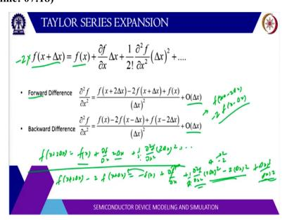
Similarly, for the second derivative you can write the forward difference. So, in forward difference we consider only the points which are more than x. So, it is f of x + delta x we can write f of x + 2 delta x that will be f of x + del x + 1 over 2 factorial
