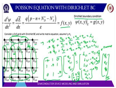
So, here you can see one example, where we have considered 5 by 5 grid point. So, 00, 01, 02, 03, 04 these are grid points. And the boundary condition is a Dirichlet boundary condition. So that means we know the value at these points we know the value at this point, we know the value at this point and we know the value at this point. So, what we have to do? We have to basically write the equations at this central points basically.
