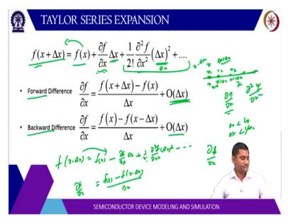
So, all of that any function f x in the vicinity of x let us say, f of x + delta x can be written as a series expansion function of multiple derivative at x. So, f x + delta x can be written as f of x + derivative times delta x plus double derivative times delta x square plus third order derivative times delta x cube and so on with some factor. So, this is a Taylor series expansion. So, we will use this to express these derivatives in terms of the values of the function.
