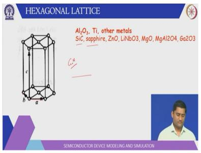
The next one is the hexagonal lattice so, in hexagonal lattice, these atoms are arranged in the form of the hexagon. So, each hexagon has a site length a another b and the height is c and the typical materials that are found in hexagonal lattice are silicon carbide, sapphire, zinc oxide. Now, some materials like gallium nitride they exhibit both the forms they may be found in hexagonal lattice or they may be found in zinc blende lattice.
