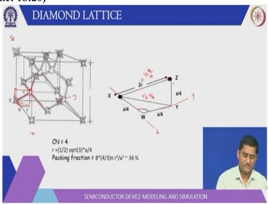
You can see further view of this diamond lattice. So, here this corner atom you can see this distance is W this is Y and this is Z. So, this is basically a Z point W point Y point. So, this is let us say X axis this is Y axis this is Z axis. So, you can think like this, this is X axis and there is a one Y axis here. So, this is parallel to Y axis, so, you can see the Y axis and then the top is the Z axis.
