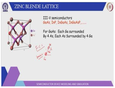
So, for zinc blende structure this is very similar to the diamond structure, the only difference I,s it is an FCC lattice with a basis of 2 atoms and the same orientation, the length is a / 4 root 3, so, x axis a / 4, y axis a / 4, z axis a / 4. The only difference is these 2 atoms are different, let us say if it is gallium arsenic, so, this atom is gallium this atom is arsenic. So, each gallium atom is surrounded by 4 arsenic atoms.
