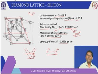
We can actually calculate other properties of the lattice if we know the lattice constant. For example, if you consider silica which is FCC with a basis of 2 atoms you can find in the literature there are tables which lists the lattice constant and the bandgap of the semiconductors. So, for silicon, the lattice constant is 5.4307 Angstrom and these lattice constants are actually calculated through x ray diffraction techniques.
