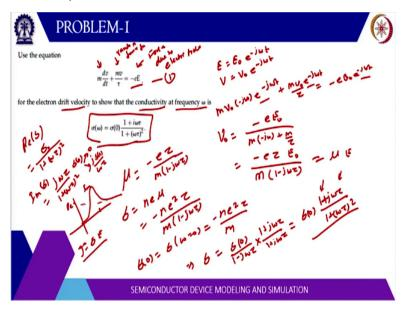
Hello, welcome to lecture number 39. So, we will take up some problems today. Use this equation governing the drift velocity of electron to show that the conductivity at frequency omega is given by the following expression. Here, it is basically a force balance equation where this is the force due to electric field then this is m dv by dt which is mass into acceleration, so which is f = ma.
