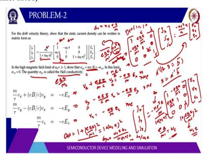
So, we can write here V x. o One more thing here you can notice the force is V cross B. This is in q times V cross B. This is an SI unit but in this problem the unit they have chosen is Gaussian units. So, this force basically becomes q times V cross B divided by C which is the velocity of light. So, this is nothing but a scaling factor relating the Gaussian unit to SI unit. So, this will appear here in this problem. So, it has to be e V by C.
