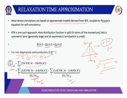
Now most device simulations models they are based on the approximate models derived from Boltzmann transport equation and then of course the driving force for these distribution function which is like electric field and all they come from the solution to Poisson equation because Poisson equation convert the charge distribution into the electric field. Now this electric field provides the impetus to change the momentum of the particles.
