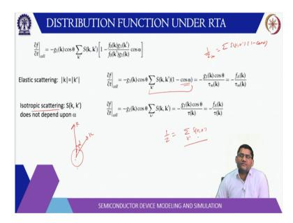
So, you can write it as this will be your tau, so tau m is 1 over tau m is sigma S k, k prime times 1 - cosine alpha. Now if there is isotropic scattering, isotropic scatter means this is your k and then this is your k prime, this alpha can be anything. So, this will cover all the equal probability it will equal probability of having angle 0 to pi and so on. So, that means if you add them all of them this term will go to 0, so in this case one over tau will be sigma S k, k prime.
