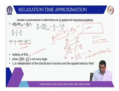
Now let us consider a semiconductor to understand what this characteristic time actually means. We are considering a very simple case where there is no special variation and there is no momentum gradient. So, that means if you piece are consider a piece of semiconductor there is no electric field so that means electric field is equal to 0 and there is no concentration gradient or doping gradient.
