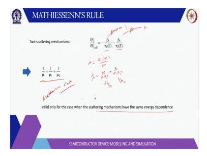
And if there are two processes so there is a process 1 and there is another process 2. So, what will happen del n by del tool will be f A by tau 1 + f A by tau 2. So, these are two skating mechanism and of course when we try mu so mu is e average tau by m. So, now 1 by tau is a scattering rate, so these scattering rate are adding up. So, what will happen 1 over mu which is m by e tau they will add up.
