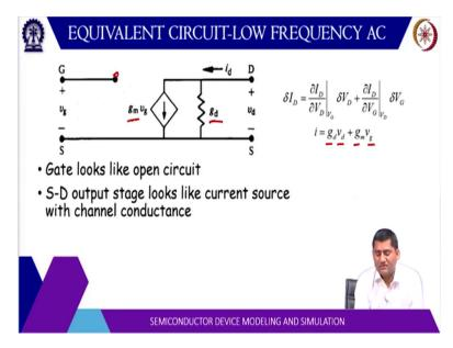
So, this is a equivalent circuit. So, here you can substitute the value for g m and g d for different regions, saturation region and the linear region. So, your I basically can be written as g d times v d + g m times v g. So, this g m is contributing the current due to the gate voltage and g d is basically the current due to the drained voltage.
