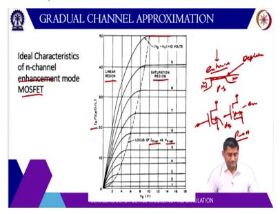
Now, this is that ideal I-V characteristic for a MOSFET. Now, here the name is written enhancement mode. So, basically there are two types of mode basically one is enhancement mode another is depletion mode. So, in enhancement mode normally the MOSFET is off. So, let us say this is your P-type silicon, this is n-type, silicon n+, this is also n+. So, it will not conduct basically.
