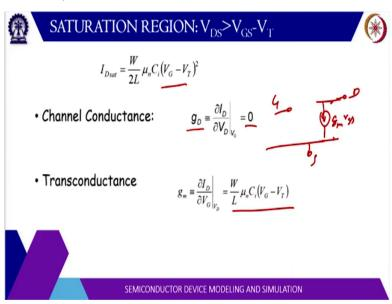
Now, in saturation region the current is constant with respect to the drain voltages only dependent on the gate voltage. So, now here the equivalent circuit will be let us say this is your gate. So, G D 0 because there is no variation of I with respect to drain voltage. So, this will be open basically then g m is del I D by del V D so that is if you differentiate with respect to VG it will be two times V G - V T.
