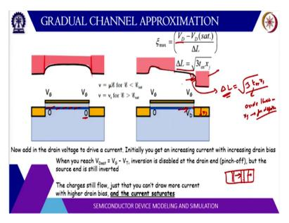
Now what happen when you go beyond pinch off? So, for a small voltage, let us say drain is close to 0. This channel is uniform when the drain voltage increases then the channel start to disappear here. And there is a small this is little exaggerated this small L is there where channel does not exist. And this actually region absorbs most of the extra electric field. So, in the length of this region which is delta L is actually pretty small.
