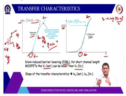
Now, we can also obtain the transfer characteristic which is basically I D versus V G. Because if you see here there is a gate here, there is a drain here. So, this is your input and this is your output, so, your V gs will be the input V ds and I D will be output. So, at the input you are applying a voltage that is V G, I D is at output. So, this characteristic is called transfer characteristic.
