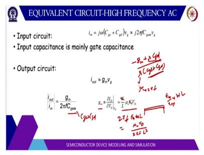
So, for input circuit we can actually calculate if you consider the circuit. Let us say there is I input here and then let us say we calculate the I output, so, let us say we sort it and we calculate I output. So, if we know the I n we can find out v g. So, v g will be I n times these two impedances C gs and C gd because this is sorted here so, and they are in parallel. So, their admittance will actually add up, so, I can be written as v g times admittance.
