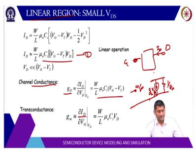
Now, if you want to get a small signal equivalent circuit. We can differentiate this let us say now considers a linear region. So, the channel conductance is del I D by del V D. So, you can look like this. This is your input gate this is output drain. So, an output current is here at ID. So, del I D by del V D is the output conductance or the channel conductance. So, this is the output characteristic.
