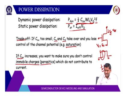
Now, another consideration in case of MOSFET is the power dissipation, of course the static power dissipation. So, if you look at the MOS structure here from the gate side, there is no current drawn. So, V gs times I gs is 0 because create current is 0 if there is a I D here. Then the power drawn from the supply connected to the drain side will be I D times V Ds. So, if there is some off step state drain current then that will be the static power loss, so, power dissipation.
