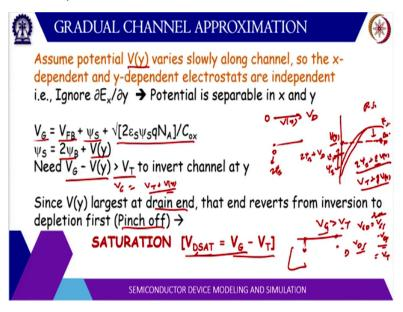
Now, let us assume this potential along the channel is varying slowly. So, at the source side it is 0, at the drain side it is V D. And individual we call it V as a function of y. So, these are the two boundary condition. Now, if you look at the channel, there are two times types of electric
