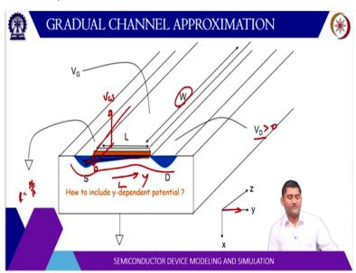
Now, the procedure that is used for calculating the I-V characteristic of MOSFET is called gradual channel X approximation. So, usually it is applicable for long channel devices for short channel. We have to make some changes but let us go ahead with this derivation so on
