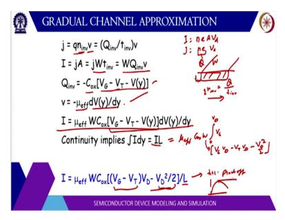
Now, along the channel region we can write the equation of current. So, current density, you know there is a total current if you recall the expression I = n e a times the drift velocity. So, j is basically divided by A so, it is n times e times V D. So, this n is basically the total charge, charge per unit volume. Because n is the carrier density is the charge on this carriers. So, this is a charge density per unit volume times velocity.
