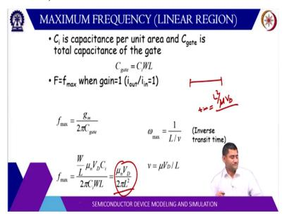
And when this is equal to 1 so, this I out by I in. This is I out by I in and there is a f here now when this gain is 1 F can be found from this one. So, F will be mu and V D by 2 by L square. Now, if you read this expression carefully, frequency will be in terms of the time it takes for the carrier to cross over the channel region. So, it will be L by V and V = mu times e. So, mu times e and e is drain voltage divided by L.
