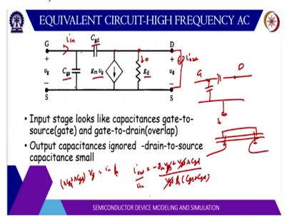
Now, at high frequencies, the capacitance layer all basically, so, you can see here C gs. C gs is the gate to source. So, if you see here, this is the gate, this is the source there is a drain here. So, this gate can have a capacitance with the source. It can have a capacitance with drain also, so, this is called C gd, this is called C gs and rest remains same g m v g and g d. So now, from where this capacitance actually come.
