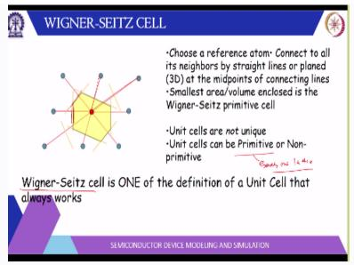
Now, there are different ways that one can formulate the unit cell in fact, one can have infinite number of unit cells and they are not unique, but there is a concept of called primitive unit cell. So, primitive unit cell is basically which has exactly 1 lattice point. So, exactly 1 lattice point so, it contains exactly 1 lattice point. So, for example, if you see any crystalline structure and this is 1 lattice point and there are nearest neighbors.
