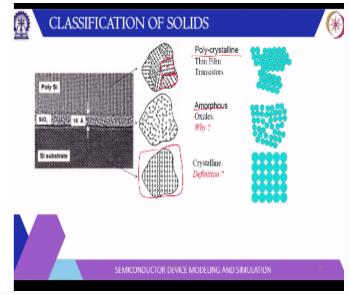
It is also possible a material or semiconductor material may not be single crystal. So, if whole chunk of material is following the pattern then we call it single crystal, but if there are blocks of single crystal like this here, this is 1 block of single crystal is another block of single crystal. So, that means it is not totally crystalline, but there are a number of crystals small crystals, which are randomly arranged.
