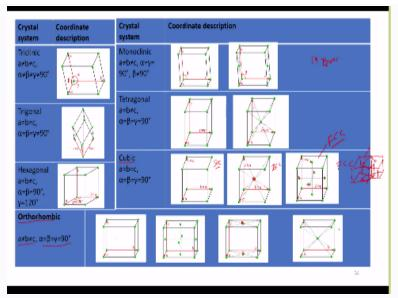
So, for example, let us consider the cubic system there are different variations of this cubic system you can have. So, this is called simple cubic SCC simple cubic crystals. So, all the corners have 1 atom each or 1 lattice point each and the side lengths are equal a, b, c all are equal then of course, you can have a 1 lattice point in the middle of the cube basically. So, that is called body centered cubic or also called BCC.
