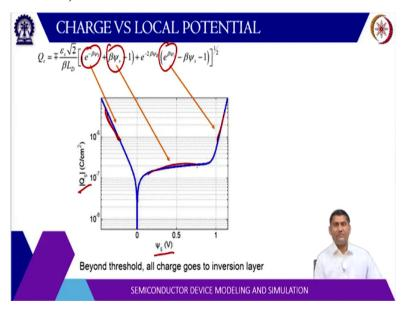
So now, let us define the other parameters that are related to MOSFET, so, this is a typical Q versus surface potential curve for a MOS structure and where we have identified the three
