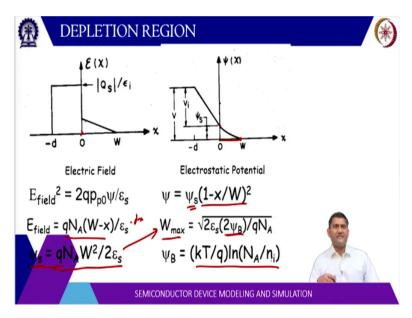
Now we can write some expressions also here. So, E square = q 2 qN A psi by E s epsilon s and if you take the, if you write in terms of the potential width, so, E field can be written as qN A times W – x by epsilon s as a function of position. At surface this x is 0 here. So, the electric field, with qN A W by epsilon and the potential will be area under the electric field. So that will be half height into width.
