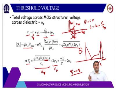
Now, the total applied voltage V T drops across oxide, so, we can write V I insulator or you can write V oxide inside the oxide + psi s the potential drop in the semiconductor. Now, inside the oxide it basically act like a there is a charge here on the metal layer. The inversion charge here is a depletion charge here this is Q n, this is Q depletion. So, this oxide is basically like a capacitor here.
