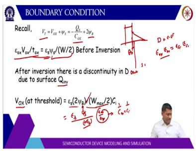
Now, let us recall that threshold voltage is Q s by C x + 2 psi B and at the interface this is oxide here. So, there is a electric field here and then there is a jump in the electric field here and then this goes like this linear. So, since at the interface if you recall that there are two regions, one is oxide, one is semiconductor, the electric field is not continuous but the flux density D the displacement flux density is constant.
