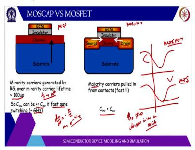
Now, you can compare these two structures one is the mass structure, so, this is metal oxide semiconductor other is MOS field effect transistor. So, here what we have done, we have made the two contacts. There is a source here there is a drain here. So, now, if you compare their CV characteristic, regardless of the frequency the MOSFET will give this curve. Why? Because now, this inverted carriers are they do not need to be generated.
