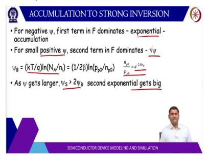
So, for a negative potential first term, in the F. So, this is the first term in the F that dominates and then this is the exponential function and this accumulation. For a small positive side, the second term which is proportional to the square root of psi. The second term beta psi s that actually dominates. And then psi B is the bulk potential that is kT by q lon N A by n i. And so, n p naught by p p naught is a exponential – 2 beta psi B.
