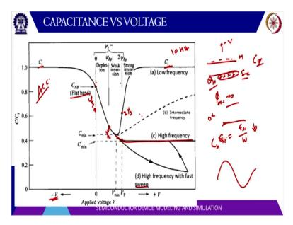
Now let us, look at this picture first so, this is voltage is negative, so that means this is the accumulation region. So, in accumulation region this is metal, this is semiconductor. So, all the holes actually accumulate here and there is a negative charge at the metal surface. So, all the potential falls across the oxide, so, this capacitance is simply C oxide or C I insulator capacitance. Then, so, this is for negative voltage.
