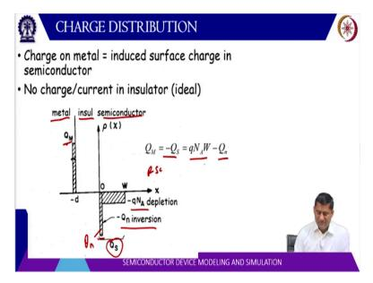
Now, if you look at the total picture, so, there is a metal here. There is an insulator oxide here and there is semiconductor here. So, in the semiconductor there is a depletion region and the charge density can be -q times N A assuming it is p-type semiconductor. Then, when there is a large positive bias here at the metal, it goes into the inversion and then this inversion charge is actually a very thin layer at the semiconductor and oxide interface.
