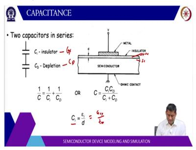
Now, if you look at the metal semiconductor of oxide structure, there are two regions here. One is the oxide here insulator one is the semiconductor. So, inside the semiconductor there is a depletion region. So, there are two capacitors series. This is the insulator oxide capacitance C ox this is the C depletion. So, when the two capacitances are series, so 1 by C is 1 by C 1 + 1 by C 2. So, if C can return as C 1 C 2 by C 1 + C 2.
