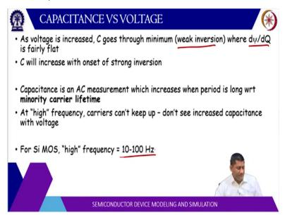
Now so, as the voltage is increased C goes through a minimum during the week inversion, where d psi by dQ is fairly flat. Then of course at the onset of strong inversion C again increases the capacitance again increases because the contribution from the semiconductor
