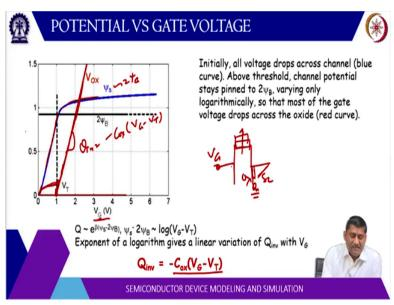
Now, this is a plot again with respect to the gate voltage. So, gate is basically this metal, oxide and semiconductor so, this is the gate voltage. So, a threshold voltage so, this is the threshold voltage here. You can see up to the threshold voltage, the voltage across oxide is almost constant but the voltage across semiconductor actually increases. Because depletion which keep on increasing here.
