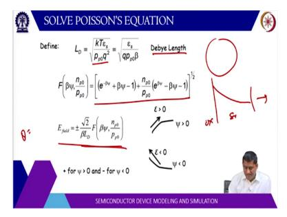
Then we can define this k T epsilon by p p naught q square we call this one as Debye length. So, it is some kind of effective length up to which the screening of the electric field takes place due to the movement of the charges because these charges can move around and they can screen the electric field. In metals these charts are large in number they move quite fast, so, they do not allow an electric field to exist inside the metal.
