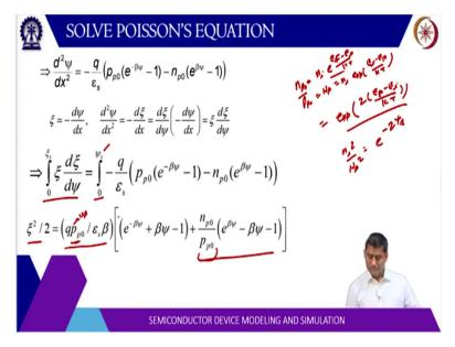
So, when we integrate it from 0 to E s, E s is the electric field at the surface and 0 is the potential in the bulk and psi s is the potential at the surface, the silicon and the insulator surface interface. So, this becomes E square by 2 is equal to if you substitute these values, you will get qp p naught. So, this is N A, q N A by epsilon beta times E to the power – beta + beta psi - 1 + n p naught by p p naught e to the power beta psi - beta psi - 1.
