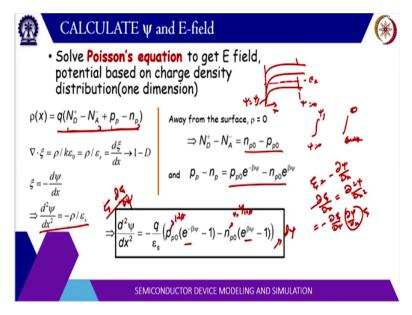
Now, this is a poisson equation, so, rho = q times the charge density which is the fixed ions N D - N A + P - N the movable charges. And if you substitute those expressions for P - N is N - P in the bulk. So, we can solve this equation with the boundary condition now the boundary condition will be basically if you look here. So, one boundary condition we can keep here where psi is 0 and one we can keep here where psi = psi s and in between this position X.
