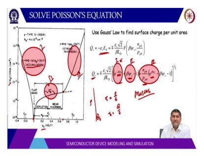
So that we can write epsilon times E. Now, you can recall basically, if you have a seat of charge, let us say some rho so, the electric field due to this set of charges rho by epsilon. So, here rho is basically charge density per unit area. So, the electric field is rho by epsilon. So, if q s is the charge density of the surface, so, the electric field will be q by epsilon.
