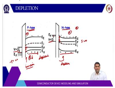
Now, if you change the polarity. So, for P-type, if we apply a voltage greater than 0. So, – qv is energy, so that means this will be negative. So, this energy is pulled down. So, all the bands are pulled down now this Fermi level is away from the valence band. That means number of holes is reduced here but this is still below E I so that means it is still P-type only. If you increase this voltage further, it is possible that this may come down further.
