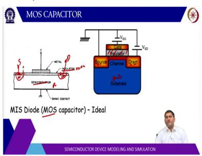
So, if you look here, there is a semiconductor then this is a small oxide layer which is insulator and then there is a metal layer. It is further enlarged here this insulator is actually, quite thin order of few nanometre or tens of nanometre and we are actually, it is decreasing year by year to have a better control on the gate. Then but this is a mass structure, metal oxide semiconductor.
