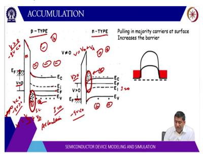
Now, what we can do when we apply the bias, so, let us say this is for p-type, so, p-type Fermi level is close to the balance band. So, now, when we apply a voltage greater than 0 then what will happen? -q v is energy, so that will be less than 0. So, a positive potential applied to the metal will lower down the energy and a voltage greater than 0 upon sorry, voltage less than 0 a negative voltage, so, -q v will be greater than 0.
