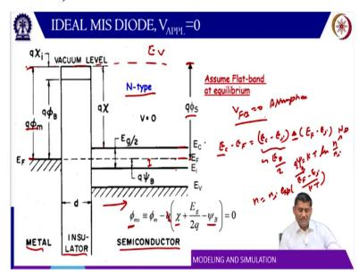
Now, let us look at their band diagram, so, this is a metal site. This is the oxide insulator. Now, this is a semiconductor site. You can see that Fermi level is close to the conduction band, so, it is a n-type semiconductor. And right now, let us assume that the Fermi level inside the semiconductor and inside the metal they are equal. So, this is not really true but to simplify our discussion to begin with, we are assuming that.
