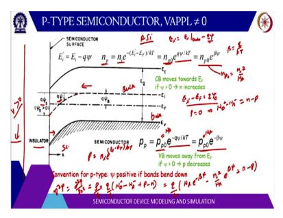
Now, how do we calculate or can we get a more quantitative expression for describing this scenarios? So, what we do here? Let us consider this P-type semiconductor E I - E F is q psi B. Then let us say there is some band bending so, this band is bending that means the E I is going down. That means on the metal side the Fermi level is pulled down here. So, Fermi level is pull down means the energy is lowered.
