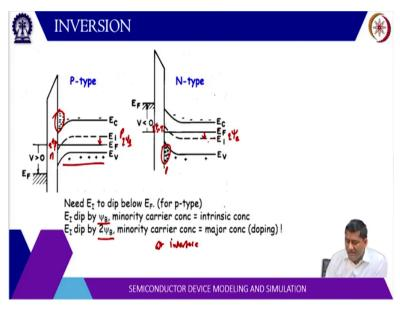
So, here is the picture showing the inversion. Now, you see here, this E F is below E I but at the surface E I is below E F. So, here it is P-type here it is N-type. So, there are lot of electrons here basically. The ion concentration is same throughout, so, this is called inversion, so only for N-type. This E I is here below E F here E I is above E F. So, this region becomes P-type.
