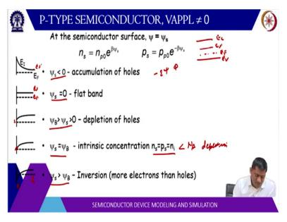
So, before we solve the poisson equation, this is the summary of the band bending. So, when psi s is less than 0 that means the potential is negative. That means energy is going down, so, energy will be -q times psi so, size negative, so, -q side will be positive. So, energy is going up actually, so, the energy is going up here. So, this is the accumulation of holes. When psi s is 0 it is a flat band, so, all the conduction band balance band all are flat basically.
