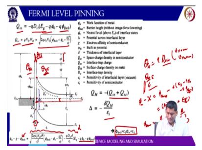
So in terms of charge, we can express it as there is a charge in the semiconductor region, there is a charge in the metal region. So this is semiconductor, this is the metal. And this metal charge, there are two charges here basically, one is at the semiconductor surface and these two charge will make up the, or they will be equal to the charge on the metal side.
