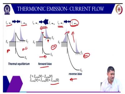
So let us look at the band diagram for metal and this is n-type semiconductor. So in equilibrium a no current can flow because we have not applied any voltage. So the current or these the flow of the electrons from metal to semiconductor will be equal to the flow of the electrons from semiconductor to metal and they will cancel out each other. When we apply the forward bias, so forward bias means this Fermi level will go up, because we have applied a negative voltage here.
