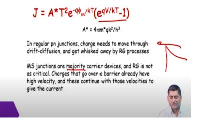
So exponential qV by kT - 1. So that will be the overall current density. Now if you notice the difference in regular pn junction charge moves through the drift-diffusion equation. So once it moves it diffuses and then there are generation recombination process in the other semiconductor. So the majority carrier slowly loses out. In metal semiconductor junction it is majority carrier dominated device.
