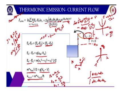
Now how do we estimate this current. So the current if you recall can be written as the charge on the electron times their velocity times the total number of carriers. So J is equal to u n times V. The number of carriers we can find out by integrating the density of state g times Fermi-Dirac distribution dE. So this will be n. Or you can also find out this by integrating f d k.
