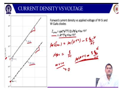
And if you plot this J versus the forward voltage, this is on log scale. So from the intercept, if you take the log of this thing, so log of J sm will be log of AT square minus q I Bn minus v by kT. So this at v equal to 0, so first you can get a slope. The slope will be q by kT with respect to v. And at v equal to 0 it will intercept as log of AT square is equal to q phi B n by kT.
