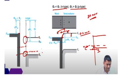
Now let us look at the metal semiconductor contact and when this contact will be ohmic. Ohmic contact means there should not be any barrier, okay? So let us say you consider a metal an n type semiconductor. If the Fermi level of metal is in between this E c and E F for the semiconductor, then it will be ohmic. When it is in this region, then the Fermi level will align and then accordingly this barrier will be very small.
