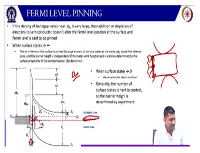
Now let us see in more detail, what is this Fermi level pinning. In case of bulk semiconductor, you can easily write the band diagram because there are no states in the middle of the band gap. So either the energy is allowed or the energy is not allowed. But at the surface, there are certain dangling bonds or these bonds are connected with some other material. So there can be states here in this region.
