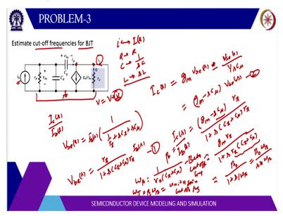
Let us look at the problem number three. Now this equivalent circuit we have already derived in the previous problem. Now the task is to estimate the cutoff frequencies for this bipolar Junction transistor. So, let us say excite this thing with a current Source a small current Source I B and we sort this collector terminal and we measure this current IC. So, to find out the cutoff frequencies we have to analyze this circuit in frequency domain.
