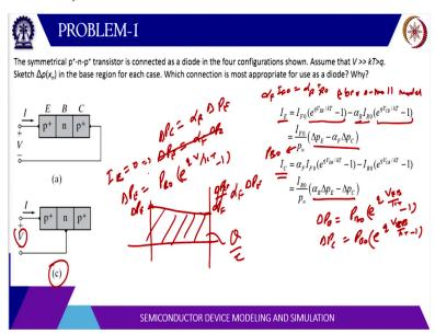
So, this is C part in case of D part this is a D part here base emitter. So, this is emitter and this is base and collector is there applied with the same voltage. So, that means your Delta P E is equal to P B naught exponential q V EB which is B applied by kT minus one and that is same as Delta P C. So, Delta p and Delta P C are equal but if you notice here the direction of current is the slope of this carrier concentration. So, from emitter current is flowing.
