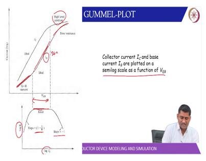
So, here IC increases and at high level injection this becomes the slope changes. So, you recall this I B characteristic for a diode in case of I B which is basically I E N there is a low level generation recombination current year then this ideal region and then there is a base resistance region. So, this is the middle region where beta is constant below the beta increases as I to the power 1 minus 1 by n and at high level injection beta decreases at 1 by I C.
