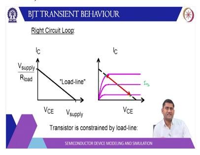
So, depending on the I B you will have different solution. So, I B is less you will have larger V CE if I B is more you will have a smaller V CE. So, transistor characteristic is constrained by the load line.
