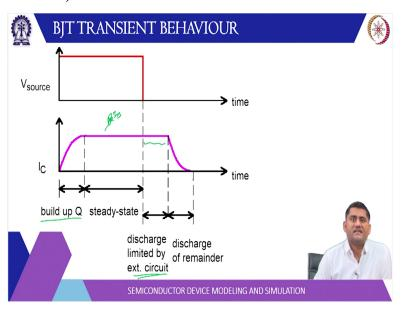
Then if you look at the transient behaviour the source is connected to the base emitter junction and when you switch on the source you apply a some forward bias I C will increase. So, the charge will be built up and then it will once it reaches ICT State you will have constant I C which is beta times I B. Then when you switch it off then initially this charge will be discharged through the external circuit.
