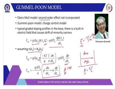
So, compared to Eber-Moll model this is a Gummel-Poon model it takes into the consideration the second order effect. So, which were not considered in the Eber-Moll model. Now Gummel-Poon model is based on the charge control method. So, if there is a gradient base profile we have slightly discussed about it the graded base profile there is a built-in electric field called E.
