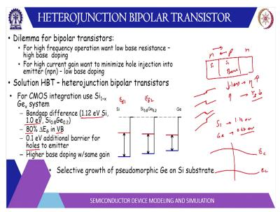
Now there are contrasting requirement in case of bipolar junction transistor for base region
