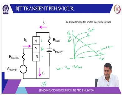
Now let us look at the behaviour to the signal variation. So, you can have transient behaviour. So, if you look at this diagram there is a base emitter voltage and there is a collector emitter voltage here. So, it is a common emitter configuration then at the common emitter you can see there is a voltage here there is R L and this voltage is V CE. So, if you plot this curve I C versus V CE you can write that V CE is equal to V Supply minus I C times R load.
