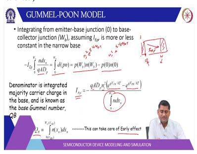
Now if we integrate this from base emitter Junction to the base collector Junction. So, let us say this is the base emitter Junction this is the base collector Junction. So, from 0 to this w. So, IEP times n by q A d is this thing dn P by dx. So, it is basically I E times n by q A d dx is
