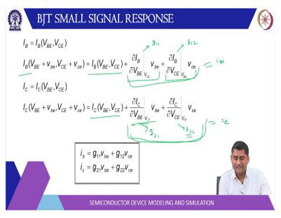
So, I B is IV DC component plus Del I by Del V B plus Del I by Del V CB times V C. So, these are basically G 1 one G 1 2 and similarly this I C this is G 2 1 and this is G 2 2. So, if
