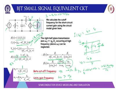
Now we can further look at the different cutoff frequencies. So, if we consider that we have applied a base current and we can find out the maximum collector current that will flow through this circuit. So, this is sorted out here and this is I B there. So, this is sort you know. So, this is also actually grounded actually. So, this I B C S R Pi in parallel with C pi parallel with C mu. So, by current division we can say that I C is a sort of (FL).
