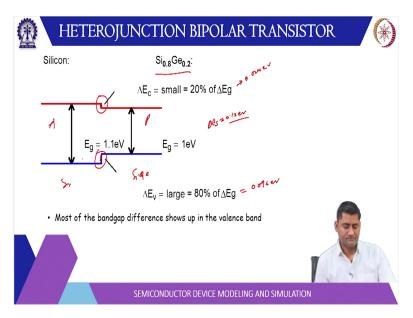
So, let us look at this Band diagram this is silicon this is silicon germanium. Now we cannot have pure germanium here because of lattice mismatch issue if we you know have too much lattice mismatch then there will be defects in the silicon germanium layer and these defects will basically tend to reduce your BJT operation and they will have some leakage issues electrons carriers will be trapped there.
