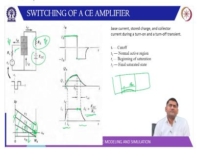
So, we can further look into the diagram this is your base emitter input. So, this is the input side this is your let us say output side the load side then when you apply a positive voltage here then some IV will be there. So, let us say we have some positive I B here then for a point of I B the charge will keep on building up. So, if you consider this region. So, the charge will actually this is the background concentration.
