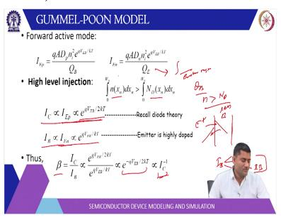
So, for forward active mode IEP can be written as you can ignore this V CB by kT. So, your simple q A dT dp and I Square exponential q V by KT by q B as a base Gummel number and similarly I E N can be written as by same logic q A d and n i Square expansor q V B by kT by q, q is the emitter Gummel number. So, this is again integral in the emitter region. Now these are the equation for the diode with a base Gummel number and the emitter Gummel number.
