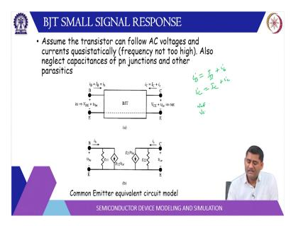
So, for a BJT lets say this is a common emitter. So, your I B is proper function of V BE and I C is function of V CE and small signal is basically each current component I sub capital B this is a total current can be written as the D C value capital I capital V plus s small I sub small b and a small signal current. Similarly I is capital Sub C capital I capitals of C which is a DC component plus a small I small Sub c that is the AC component this can be written like this.
