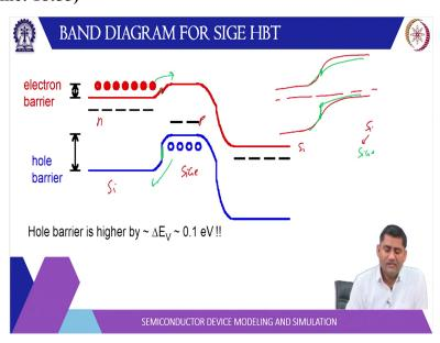
So, this is your silicon this is silicon germanium this is N type this is P type. So, in case of equilibrium the ferment available is same and this will go like this will be somewhere here. So, if both were let us say both were silicon ok but if this is silicon germanium that means different colour here I say this is silicon Germanium. Now the bandgap is not this much. So, 20 percent falls across here 80 percent falls across here.
