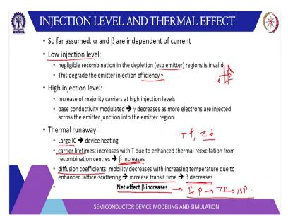
There are some other ah considerations similar to the PN Junction diode we can see here at low level injection because in the derivation we assume that in the deeply region there was no recombination generation and especially at the base emitter junction because this is forward bias. So, there will be some recombination and that will degrade the emitter injection efficiency because the holes that are coming from the emitter.
