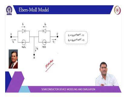
So, this is very simple model and you can replace you can write this equation maybe write a Matlab code ok to get the front IC BC curve or IV DB curve. So, different characteristics for the Mosfet for the BJT can be obtained using this model. So, this is basically coming from solving the meiotic carrier diffusion equation in case of BJT with all the assumptions that we have stated.
