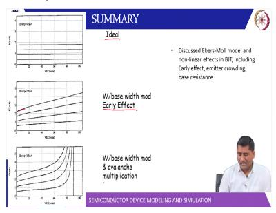
So, in summary we have discussed the Ebers Moll model and we drive the condition that I C versus V EC is constant for ideal when it includes the base width modulation or early effect it actually tend to increase sub linearly and then if you include the Avalanche effect. Then some this breakdown can be observed at certain voltage and then of course we have discussed other parameters like emitter crowding and the base resistance effect, thank you very much.
