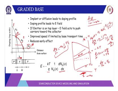
Another technique that is used or rather there are two ways of getting the the doping profile one is diffusion other is iron implantation. So, in iron implantation we can be more precise and we can control the dope and distribution profile in case of diffusion it is thermal thermally controlled process. So, we do not have much control on the profile because if you apply the heat treatment it will follow certain Gaussian or Winner function profile.
