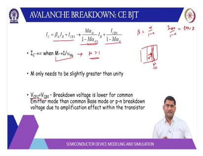
So, if you recall the expression for I C is beta times I B plus I CO and beta is Alpha over one minus Alpha and Alpha is the base transport factor now what is happening here Alpha is a base transport factor and then at this reverse bias under breakdown this is a multiplication. So, what is happening here you instead of alpha you are getting m alpha. So, if you replace this Alpha by m alpha.
