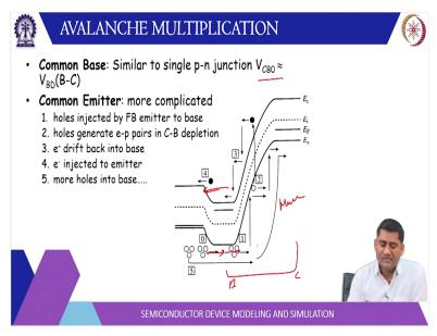
Common secondary order effect we can see the breakdown phenomena. So, we have already discussed a breakdown phenomena in case of PN Junction. So, when PN Junction is Zero's bias. So, this is a base collector Junction it will break down a certain voltage. So, that is for the common base and we call it V CBO that will be same as the breakdown of this base collector junction in isolation but in case of common emitter.
