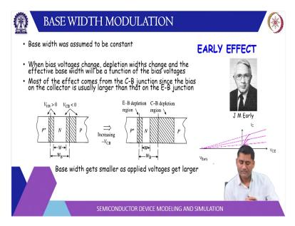
So, these two phenomena have to be explained. So, in the model in the beginning we assumed this base width was constant but your base character is forward bias. So, the depletion width for the base collector base emitter Junction is usually small. So, it is not a point of concern but the base collector is reverse biased. So, here the base collector Junction depletion width will increase especially if you increase the reverse bias.
