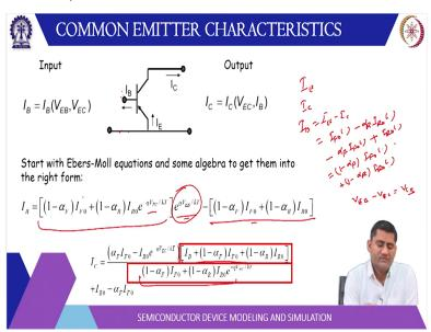
And if you plot this characteristic so, your I B versus V E B as you change the V E C if you change the V C here because V C is not small it is significant. So, this term will change basically. So, for higher V E C the current will decrease and that can be understood like this
