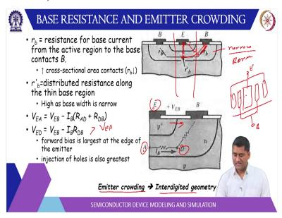
And another phenomena is the base resistance because base is actually narrow here and is doping is limited it cannot be as high as emitter. So, it has some resistance and if you see this region the cross section region here it is away from the base contact. So, the base current actually has to travel something like this. So, there is a base resistance and there is a base spreading resistance. So, the potential difference between these two terminals and these two terminals is different.
