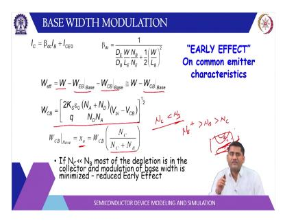
Now in case of common emitter also you can estimate the width of the depletion region. So, W is basically W the natural width of the base minus from the emitter side depletion region minus depletion region from the collector side. So, because emitter side is forward wise this is small we can consider the depletion weights on the collector side. So, actually in the base due to the base collector voltage and this is the expression you can recall from the diode.
