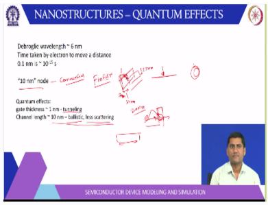
Let us consider this 10 nanometer node today's MOSFET technology. Now, these names are basically commercial once. So, this 10 nanometer node name is a commercial one length of the channel or any physical parameter. This is a convention adopted by ITRs. So, for example, for 10 nanometer node by Intel it uses actually FinFET a structure. So, it is again the FET structure field effect transistor, but instead of having a channel some fins are there which act as a channel.
