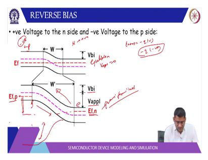
So, this is the typical band diagram this is under equilibrium when there is no applied. So, V applied is zero here. Now if we apply a reverse bias. So, reverse bias means this is P side this is N side. So, in Reverse bias P side is negative N side is positive that means a negative potential here means the Fermi energy will be more because energy is minus q times V. So, V is negative. So, minus q times a negative voltage will be a positive.
