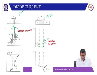
So, they both give rise to the same equation. So, in summary we can write that for a PN Junction when it is forward bias. So, this is the forward bias holes are injected from P side electrons are injected from N side. So, from this you can also tell the whole concentration is large. So, P side is highly doped compared to N side and then there is a you know carrier gradient. So, that tells you the diffusion current the slope at this boundary of the depletion region.
