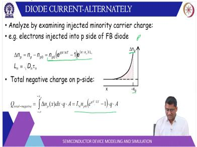
There is another simpler way to calculate this current and that is called basically charge zero charge conservation. So, you can look on let us say on P side. So, on P side these are this is the electron profile that we have calculated that n p naught exponential q by kT this excess number of electrons. So, this is in excess to the actual minority carrier concentration times exponential x + x p by L n.
