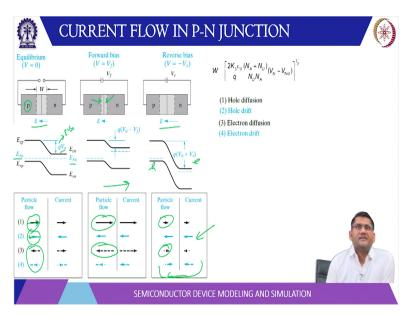
Now here you can see the summary. So, under equilibrium the built-in potential is the q times V bi written as V naught here and there is a single Fermi level. So, E FP and E FN they have a silicon cite and you can also notice the particle flow. On P side holes actually diffuse. So, this black line is the hole diffusion and you see the direction of electricity it is opposite. So, hole will drift in opposite direction.
