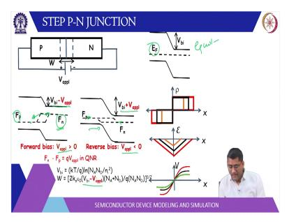
So, this depletion which is now basically functions of the applied voltage. So, in equilibrium this difference is V bi in case I applied forward bias this barrier reduces and these Fermi levels separate out. So, in equilibrium there are single Fermi level in case of forward bais we have 2 Fermi level F N and F P and F N is above F P. So, that means another thing you can notice here because Fermi level is tells you the probability of finding electron.
