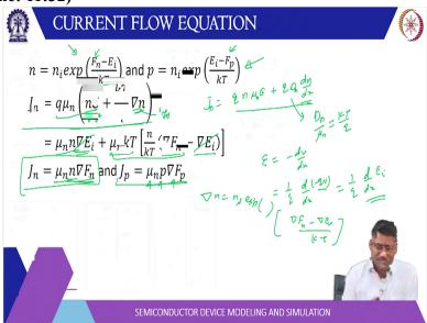
Now this equation we already know there are 2 components here one is the drift another is the diffusion. If you recall that J is q times n times mu times E is the drift Plus q times D times D n by dx the subscript n here. So, we skip 10 here this is the current density for electrons this is for 1D basically. In 3D this D n by dx get replaced by gradient of n. Now there is a relationship between this d and mu so this is called Einstein relationship.
