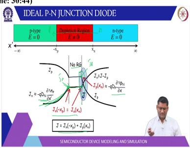
So, when you combine the 2 this is the mind to carry diffusion equation on P side this is a magnetic array division on equation on N side. So, on N side holes are in minority on P side electrons are in minority. So, number of electrons that are injected here less is Delta n number of holes that are injected is Delta p. So, when you solve this equation basically you will get some exponentially decaying terms basically.
