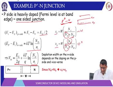
So, if doping concentration is higher you will expect a higher electric field and now we can consider one example of one sided Junction. Now one side is Junction is basically where one side is heavily dropped compared to other. So, you can take P plus N or P N plus. So, when you write plus here that means this region is highly doped. So, more than ten raised to power nineteen and so on.
