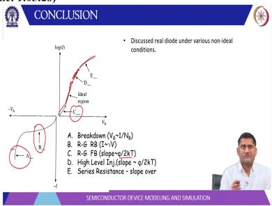
So, in summary we can say the IV curve of PN Junction consists of several regions where a is the breakdown region. The mechanism can be Avalanche breakdown which has positive temperature coefficient it can be Zener breakdown which has negative temperature coefficient then there is a recombination region the current due to the sorry generation this is due to generation.
