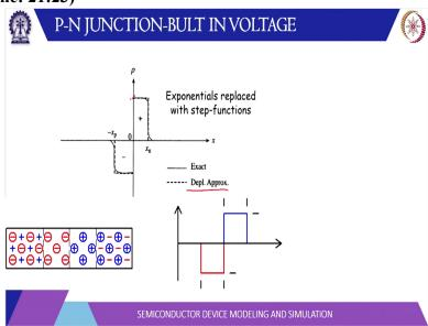
We can find other parameters also, now just to remind that we are assuming step Junction profile. So, we are basically assuming the depletion box with a abrupt transition but in reality it will not be abrupt it will have some curvature so that we will discuss in one of the problem. But right now we will move ahead with this depletion approximation. So, by solving the exact equation is also possible to find out the exact profile.
