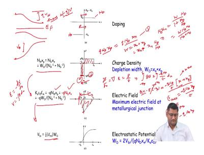
So, going ahead with the depletion approximation let us calculate other quantities. So, this is basically the doping. So, N d on the electron side or N type site and N a is on the whole side or P type side. Now because of the movement of the carriers holes, so, the holes had moved from right to left electrons are moved from N type to P type and that has basically uncovered these negative ions receptor lines and these donor ions.
