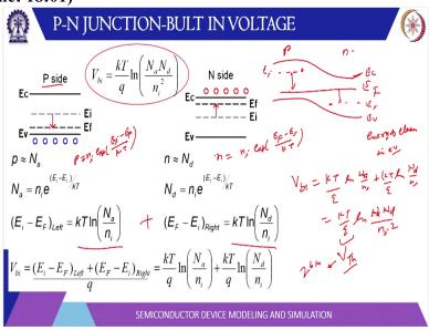
Now let us have a further look at the Venn diagram of P-N Junction because in equilibrium these Fermi levels align basically. So, that means initially on the P side permeable is below the intrinsic level by an amount called kT log N a by N i that you can easily find out from this expression for the carry concentration that P is equal to N i exponential E i minus E F by kT and similarly N is equal to N i exponential E F minus E i by kT.
