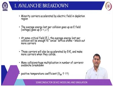
Now these magnetic areas are accelerated or the electric field. So, this we have already discussed and at high field of course this V equal to Mu it does not apply but in the linear region up to certain point this is true that V is equal to Mu a and then of course when there is a critical electric field the average energy lost is in enough to ionize the lattice atoms or knock out the electron.
