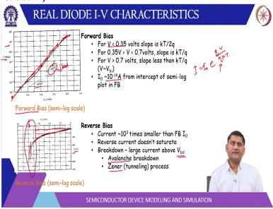
This is the; if you consult some data sheet for a typical diode you will get characteristic like this. So, this is forward bias. So, in forward bias in the region around 0.35 to 0.7 this slope is q by kT. So, that means here the diode is behaving like an ideal diode below this region the slope is less above this region also slope is reduced. So, this can be approximated by q by 2 kT. So, for voltage less than 0.35 and greater than 0.7 of course it can be again not kT by q but some other slope.
