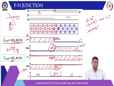
So, here you can see P type semiconductor N-type semiconductor. Now here we have shown the comparative band diagram and the charges without actually connecting them. So, they are still separate but the band diagrams are shown side by side. Similarly you can see these positive ions are immobile these negative ions are immobile and then these holes and these electrons are mobile. So, if you look at the charges.
