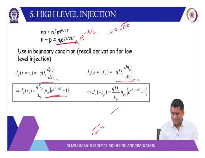
So, this is the case that happens between the point three five to point seven volt then at high level injection of course you can directly write this same thing n p product is n i Square exponential q V by kT and you can substitute this equation for the minute carrier diffusion in the quasi neutral regions and then of course when you calculate the diffusion current q dp times dp by dx for N site because holes are minority there and for electrons on P side you can write q dp times dn by dx.
