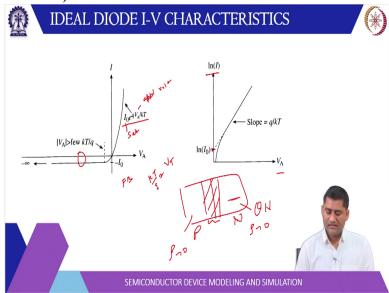
Then we develop this thing using charge conservation model. So, in summary we can write that for ideal diode current is given by some I naught times exponential q V by kT where I naught is the saturation current or reverse saturation current and V is the applied voltage and T is the temperature k is a bolt span constant and q is the charge on electron and kT by q is non (()) (34:25) called thermal voltage V T.
