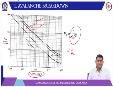
And this is the curve which relates the breakdown voltage versus the doping in case of these materials gallium arsenide, silicon and germanium and as we drive that it is roughly proportional to one over NV. And if you fit it with the experimental value you get around power 0.75 and with the increasing doping the breakdown voltage is actually reducing. Now this doping is on the lighter doped side.
