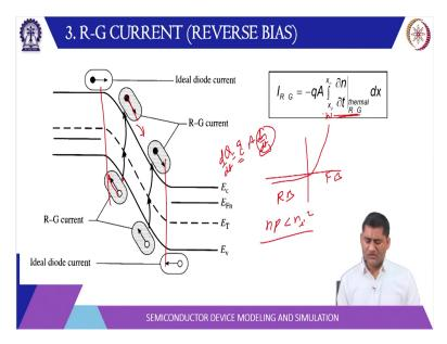
Now let us look at the IV curve of a P-N junction diode. So, you can recall here the IV curve basically look like this for ideal diode. So, in forward bias exponential in Reverse bias it is a constant and that was the case when we ignore the generation recombination in the generation recombination in the depletion region. Now in real diode there is a certain amount of generation recombination in the depletion region.
