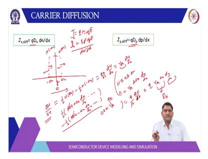
So, when these mobile charges will move then the charge may not be zero in the vicinity of interface. So, let us look at the diffusion current we already know that we have discussed the drift current. So, drift current is given by q times N times V or is given by mu times electric field and this is for electron similarly for holes drift current is q times P times mu times E. So, this is Mu P this is Mu N where mu is the mobility and that concept we have already discussed.
