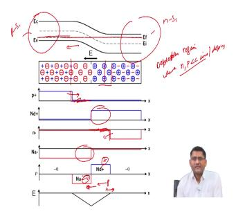
Now when we combine them the Fermi level has to be constant at equilibrium because we have not applied any bias and this also means that current flow has to be zero. Then accordingly the conduction when valence band they are bending near the interface and away from the interface you see it is again like undisturbed P type semiconductor. Here it is again undisturbed N-type semiconductor and because of this movement of carrier so, wholesale moved from here.
