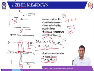
Now the second mechanism is the Zener breakdown in case of Zener breakdown the mechanism is the tunnelling. So, if you look at this picture here let us say this is some potential barrier with height V naught and the barrier thickness is d. So, this particle if thickness is small comparable to the de Broglie wavelength of this particle there is a finite probability that this electron can go over this barrier even though its energy E is less than V naught the the energy of the barrier.
