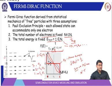
Now, in this lecture, we will learn how do the states are filled by electrons as we know electrons are fermions and therefore, they follow this function called Fermi Dirac distribution function. So, this is basically derived from a statistical mechanics of free particle with the following assumptions. We have this Pauli Exclusion Principle which actually allows that each state can accommodate only 1 electron and if second electron is there, it must have an opposite spin.
