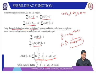
Then we can use other 2 constant that sigma N i = N there is a total number of electrons that is conserved and sigma E i N i is the total energy and of course, if you differentiate with respect to dN i, so, this is sigma dN i will be 0 because, N i is fixed so, dN i so energy is also fixed, so, dN i total is also 0. So, sigma E i dN i is also 0. Now, when we use these 3 equations and that method is called method of undetermined multipliers.
