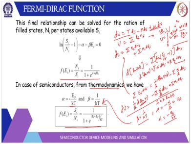
And using the thermodynamics, we can evaluate these coefficients which are alpha and beta this is the Fermi Dirac distribution function with some coefficient alpha and beta and from thermodynamics we find that alpha comes out to around minus E F i kT and beta comes around to be 1 / kT and when you substitute you get this expression. So, let me elaborate about these thermodynamics, what we can say that change in the internal energy is equal to Tds T is the temperature, s is the entropy minus Pdv.
