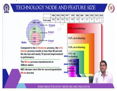
So, here you can see the wafer sizes, the 6 inch wafer which is 150 mm the 8 inch wafer and that 12 inch wafer people did not go beyond 12 inch wafer, because if you increase the size of the wafer they there are some other defects that come into the picture. So, because of this large size, they are can be going of this wafer and the defects section not be controlled. So, well they are and also processing of this large wafer is also difficult. So, this 300 mm or 12 inch standard is optimum.
