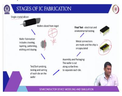
Just to give you the overview how these devices and the integrated circuits are then coming to the market. So, first of all, we start with a single crystal silicon, there are methods to grow these crystal silicon and those Wellsky method and then these wafers are sliced from this ingot and then this wafer is actually is quite big. So, you know several DICE has created out of it. So you can have one dice maybe of this size. And then each dice is tested for functionality.
