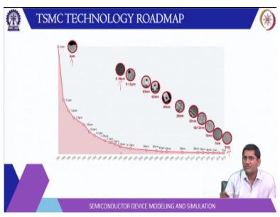
This is a pictorial representation of the technology roadmap by TSMC. So, here you see in 1988, this was 3 micron and then this is 180 nanometer in 1999 and in 2009 19 it is already 5 nanometer. So, these are the typical feature size that are scaling. Now, beyond this if you see you
