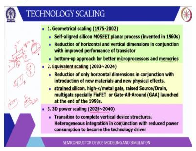
So, this scaling can be divided into 3 eras of scaling. So, one is called geometrical scaling, which was dominant from 1975 to 2002. So, in the geometrical scaling the most FET that were fabricated, they were using this self aligned planner process, which was linear invented in 1960s. And of course, the horizontal and the vertical dimensions of the transistor well reduced and this approach was called bottom up approach.
