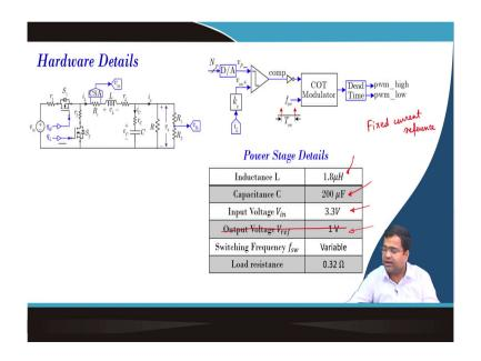
So, now we are going to consider some hardware results. So, in this hardware result, we will take the power stage and we have an inductor this thing we have discussed multiple times. The input voltage will vary to show, the output voltage we are using as a fixed reference.
