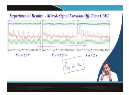
Because if you see from 2.5 to 2.25 and 2 volt 50 percent your current loop is perfectly stable. Since we are using constant off-time control where the ripple current is more or less the same. You see the 3 cases. So, the output voltage you can see they are more or less regulated.
