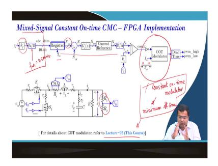
And if we consider this DC-DC converter in the buck converter then we have discussed that this part is our ADC voltage feedback gain, because we have this resistive divider. Then ADC data is sent here we are using an ADC clock which is a 25 megahertz clock. This is a very high-frequency clock I would say.
