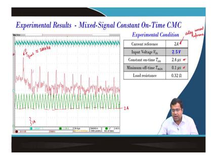
So, if we now go to the next, first we are taking the current reference to 2 ampere because it is a valley current. It is a valley current reference because it is constant on-time control and this is the experimental result.
