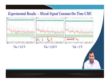
Now, we want to compare 2.5 volt 2.2 volt, and 2.2 volt. So, you see the current ripple. So, the delta is delta iL decreasing in this axis if the input voltage and since delta L is decreasing. So, the frequency is also increasing, and what is decreasing? So, here input voltage is decreasing.
