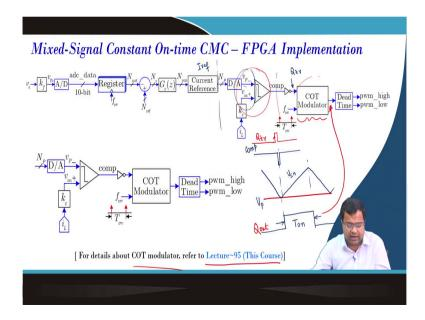
So, what is in this case I mean if you consider the constant on-time control. How does it work? So, suppose we have this current reference and this is our inductor current. When it hit the current reference then the on-time is started. Once the on time is elapsed then starts falling and this is the methodology.
