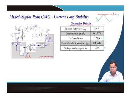
So, I will say instead of the controller it is the hardware details where we are using a reference peak current. That means, we are applying a peak current that is 3.4 ampere and we are comparing the inductor current with this peak current; that means, this is the inductor current we are comparing. So, 3.4 ampere is the current reference, but that is a physical current reference, but actual implementation because there will be a current loop gain and etcetera.
