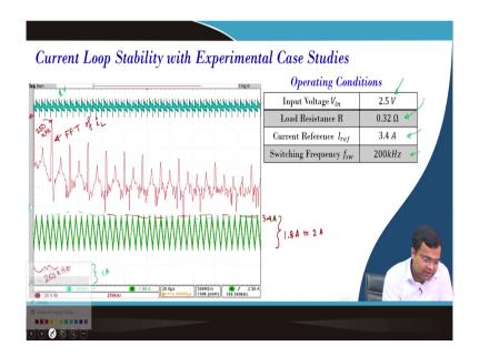
Now, I am showing the first experimental case study where we are setting the input voltage to 2.5 volt, and the load resistance is 0.32 that I have told. The peak current reference is 3.4 ampere and the switching frequency is 200 kilohertz. And if you see the experimental result and you see this division is 1 ampere for the current and the voltage if you see 1, 2, 3, 4, 5 it is almost 1 volt.
