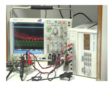
So, now we have placed the 0 frequency here. So, you can see there is a spectral peak at 200 kilohertz. Because this length is 250 kilohertz and this one is 200 kilohertz. So, that is our switching frequency that is the fundamental component and then there are harmonics.
