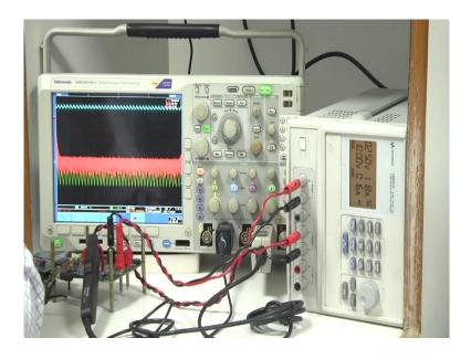
Now, we are coming to the actual demonstration. So, this is the power supply where we have two the first channel. This is the second one is for powering different IC you know ADC, DAC, and all and the first channel is our actual power input.
