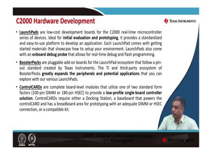
Now, we will look at each of these hardware urban platforms in a little bit more detail. The LaunchPads, LaunchPads are the low-cost development boards used for initial evaluation and prototyping. We provide a lot of software and examples to run on the LaunchPads and also the LaunchPads have onboard debug probe that allows you to do real-time debugging and flash programming.
