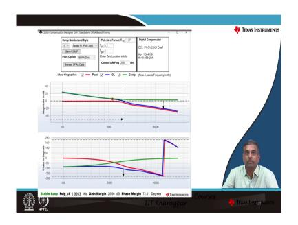
So, this is a pictorial view of how the composer looks and you can see that we can see the magnitude and the phase; also, we can see whether this loop is stable we can see the gain margin phase margin. We can also choose the type of compositor we want and also this helps you to quickly retuned your algorithm and rerun it again and again and check your stability. So, I will now show you an overall flow of how you use all these tools for your digital power design.
