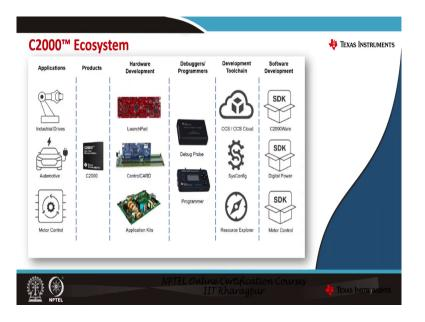
The C2000 ecosystem is very broad in the sense that along with our devices, we also provide the hardware development platform, which are the LaunchPads, control cards, and application kits. We also provide a set of debuggers and programmers to enable software development and we provide our development tools chain like the CCS SysConfig and resource explorer to create your software.
