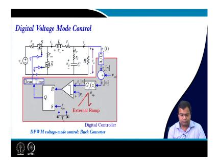
So, this is the overall architecture of the DPWM block, Digital Pulse Width Module is a voltage mode control.
