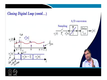
And this conversion time actually if we want to draw this timing diagram. That means, this is the digitized voltage; that means, this is the digitized voltage digitized output voltage. So that means, it will be a number, so if it is an 8-bit ADC then an 8-bit number, and so on.
