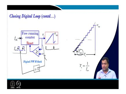
So, in summary, that means, if you use just a counter it can be a modulo counter, it can be a free-running counter. In the case of the free-running counter, you have to compare it with the upper limit and we can suitably adjust the switching frequency just by changing the upper limit if we keep the sampling clock the same.
