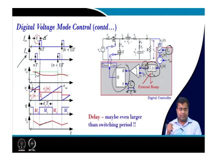
And if we show the waveform overall waveform. You know where it is the fsw clock which is a switching clock. And again we want to recall you know what we have discussed, I think lecture number 7, yes. Modulation technique this voltage mode control analog control is a trailing edge modulation.
