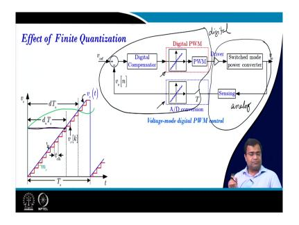
So, this block I would say, from here to here is our digital and these blocks are analog ok. So, here there are two places where you need to consider quantization. One is the ADC resolution where the quantization will come into the picture, another we are using a counter base or maybe other architecture of DPWM where it will be a staircase.
