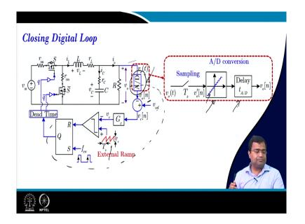
If you want to close the output voltage loop, then first thing again we want to the first thing is required we need to digitize this voltage signal. That means this is the output voltage. Again we may not use a straightaway ADC we may have to use it as a resistive divider or op amp buffer circuit.
