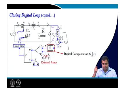
So, now, again the next part when you have a digital signal here, naturally this compensator has to be discrete time. That means, this compensator will be sitting on the digital control platform, which can be a microcontroller, ASIC, FPGA whatever.
