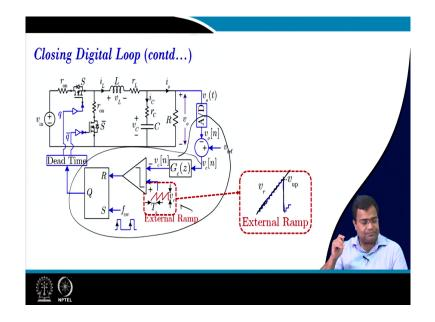
So, next to the ramp, since we are all talking about digital because so far all these signals are digital ok, so these are digital. So, naturally, this ramp should be digital and how do I generate this ram for this ramp? A very easiest way you should use a counter as if the counter is just kind of incrementing right. So, in the counter state keep on incrementing again you reset the counter.
