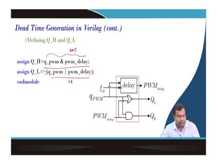
So, in one line you can write; that means, assign Q H this is in data flow modeling where which represents the AND gate. And this is a not of OR operation. So, this is the OR operation and this is the AND operation ok. So, AND operation or operation and this is the invert; that means, you are complementing this.
