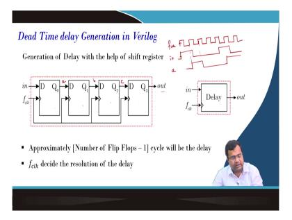
That means if you write this Verilog code delay generation. So, the delay has to use a shift register; that means, there is a clock whenever this edge clock comes this signal is propagated
