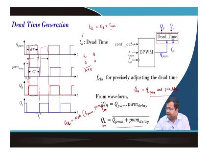
So, let us say you know. So, for clock frequency, we can use the clock frequencies which means the resolution of this td this td will be some N number of delay into the T clock time
