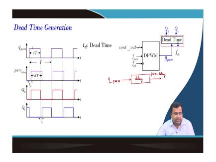
So, how to generate this dead time circuit? If you go we are delaying this PWM signal; that means if i pass this q PWM through a delay block. So, delay block and this delay should be customizable then we are talking about PWM delay. So, that signal is named and you can see it is delayed. Now if you look at this waveform how do you synthesize it? So, QH and QL how it is generated? td that is the dead time ok.
