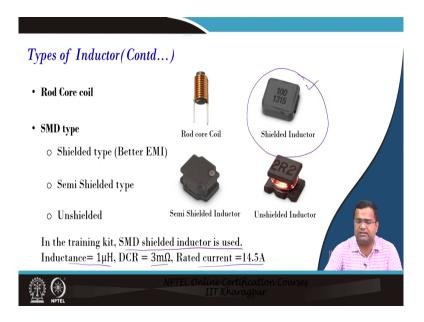
Then rod core coil SMD type shielded type. So, if you go for SMD type surface mount type then it can be shielded for better EMI and this is what we are using in our course shielded type. Then semi shielded or it can be unshielded in this training kit we are using a shielded core; which means, the inductance value of 1 micro henry, DCR around 3 milliohm, and we rated the current as 14.5 so; which means, around 14 ampere current. So, this is the core that we have selected.
