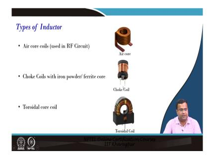
Now the type of inductor can be an air core coil ok and these are used in RF circuits, then it can be a choke coil with iron powder or ferrite core and this can be this is a choke coil or it can be the toroidal core coil. So, we often use you know these first two cores for a power inductor.
