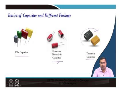
Now, if you go to the capacitor we know the capacitor can be a film capacitor or it can be an aluminum electrolyte capacitor, which is a very common capacitor or it can be a tantalum capacitor. So, these are a bit expensive, but all these are SMD this is SMD type this is through the hole you know and this aluminum capacitor here is you know through the hole, but it can be SMD also.
