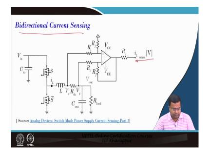
Now, the bidirectional current sensing: So, this is something like a full current sensing in this case; that means, we are putting a shunt; that means, the resistance in series is the inductor
