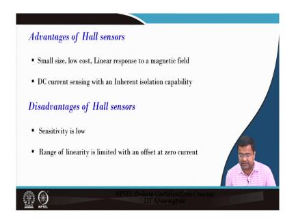
So, the advantage of the hall sensor; is the hall sensor can be small in size, low cost, linear response to a magnetic field, and DC sensing with an inherent isolation capacity. Disadvantage; it has a low sensitivity and the range of linearity is limited.
