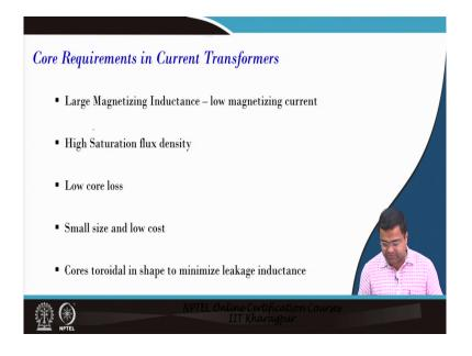
And the requirement of the current transformer, the current transformer should have a very high magnetic inductance so that the low current magnetizing current should be very very low. And the saturation flux should be high so that it can swing you now to large extent. The core loss should be reduced and also size and the cost should be reduced. And then it is if you take a toroidal kind of shape then you can also reduce or minimize the leakage inductance.
