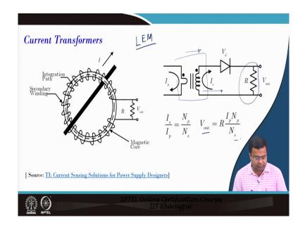
So, this is a current transformer, in the current transformer one of example is the LEM current sensor which is the current transformer. So, the primary side coil actually whatever current is passing through that goes to the secondary side coil. And the secondary side there is a diode and now how it works; that means, it is using a current transformer principle and the step-down ratio is quite small the current.
