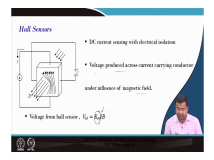
And this magnetic field will influence the voltage produced across this sensor. This voltage produced across the sensor will be influenced by the magnetic field; that means if the magnetic field changes the voltage will change and that will capture the current flowing through this conductor.
