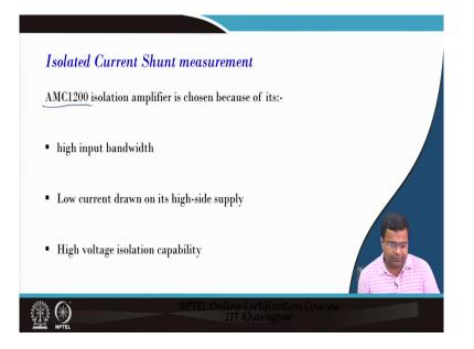
So, typically AMC 1200 is one example of an isolation amplifier it has high input impedance, low current drawn, and then high voltage isolation capability.
