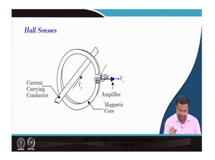
The hall sensor is another you know kind of very important sensor, where is the hall sensor principle? So, the hall sensor works in the principle that it has its voltage this is a sensor hall sensor, and if you keep this sensor close to the magnetic field, because if the current is flowing through this path and then it will create a magnetic field.
