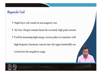
Now, so, this Rogowski coil is a single-layer coil owned on non-magnetic core and air core output I mean this flux; that means, the air core output remains linear for extremely high peak current. And this is useful for fast transient current even the pulse current.
