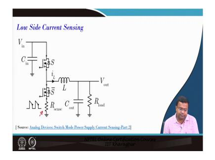
But, in many applications the low side current sensing let us say in buck converter, you can implement analog low site current sensing you can implement valley current mode control. But in digital even by sensing low side current, you can implement peak current mode control by using fully digital current mode control where the rising slope can be emulated inside the digital controller. So, many possibilities exist.
