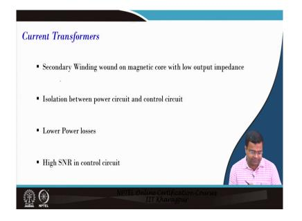
So, the current transform on the secondary side is one so, it has it should have a low output impedance and it gives you isolation between the power circuit and the control circuit. And the power loss can be reduced in this case the transformers should have a very low power loss and this kind of sensor also gives you a high signal-to-noise ratio.
