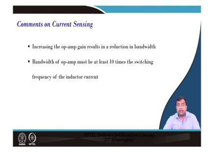
Then it is increasing the op-amp gain result in a reduction in bandwidth. That means, what way is the best? If we put a large resistance then the losses will be more and that is not acceptable because it is in the power part. But if you take a very small resistance then you need to use a high gain of the op-amp. So, you can get sufficient voltage corresponding to the current and high gain if you increase the gain of the op-amp then the bandwidth can reduce, so you have to be very careful.
