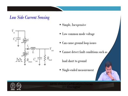
Like low-side current sensing in low side, you can put a resistance just below the low-side switch and you can simply take it as a ground reference. So, it is a low side sensing; which means, low common mode voltage it is very inexpensive in many applications you use but again you have to be very careful about the parasitic of the resistance.
