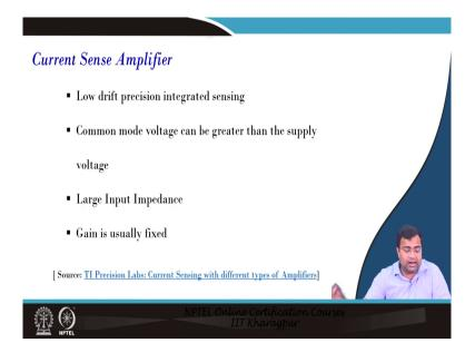
Or current sense amplifier generally has a low drift precision integrated circuit; the common mode voltage can be greater than the supply voltage. Large input impedance and it can have a fixed gain, it is unlike that you know a regular amplifier where the gain can be adjusted here it is a gain is fixed.
