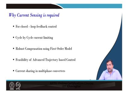
So, why current sensing is required? For the closed loop you know the feedback control cycle by cycle current limit because we know about the current mode control you know cycle by cycle current limit. Then we also have robust compensation because, if you use a current mode control, then we can virtually represent that the converter like you know you can inductor will become virtually a control current source.
