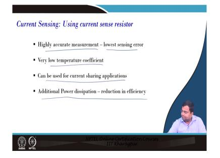
Then using current sense resistance the accuracy because very highly accurate with a lower in the lowest sensing error. But a very low-temperature coefficient, but it can be used for various applications it has an additional power loss and you also need a separate differential op-amp and all this arrangement.
