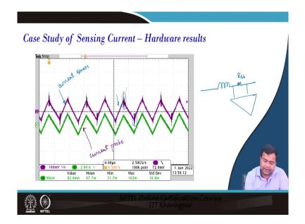
And this is the waveform of the board that we will be you know showing our NPTEL course harder case where the blue one I mean. So, green one here the green one this is the probe current probe this is from current probe sorry current probe, it is coming from the current probe and this is coming from the sensor current sensor and we are using this is the inductor current.
