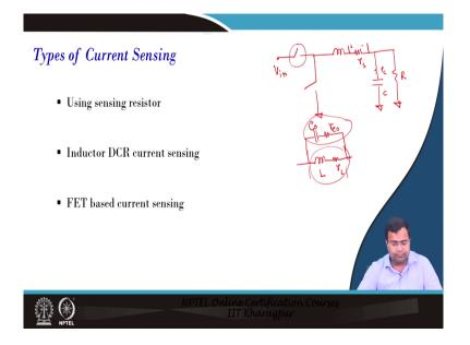
So, typically the current sensing technique that you have is a sensing resistance, right? You know if we take an inverter like an inductor suppose we are talking about a buck converter. So, suppose this is our buck converter and this is our input voltage, now we have this inductor right. So, one way we can put a sense resistance here and then we have a capacitor and this is our inductor I register load resistance.
