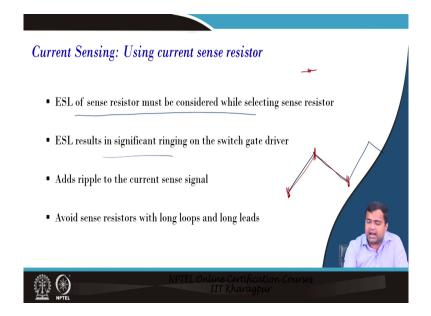
Now, in current sensing using sense resistance the ESL effect must be considered as we have discussed because it will introduce spikes. ESL can result in ringing at the switch node particularly when there is a turnover; that means if you have this kind of thing. So, it can
