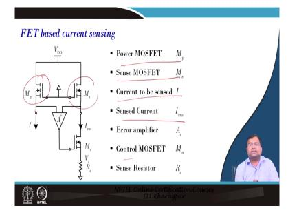
Another way is a FET-based implementor; which means your switch. So, if you use a power switch then you can use you know this is the power switch, but you can use a mirror of the power switch; that means, you know these are the power switch is M p, the sense MOSFET is M s, then current to be sensed that is I, but you can create a mirror that senses current error amplifier control.
