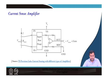
So, for the current sense amplifier typically we can use a dedicated current sense amplifier with proper biasing and all.
