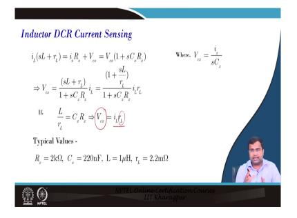
How does it work? So, if you obtain this you know all this calculation it turns out that the actual inductor is the voltage across the capacitor which is a V cx this voltage across the capacitor will virtually become i L into r L, where r L is the DC resistance of the inductor if you can match the time constant ok.
