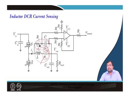
Then the DCR sense we have discussed because the inductor has it is own internal DC resistance and we are putting an external resistance as well as a capacitor. So, here the time constant of this branch should match the time constant of this branch, and then we have to take the differential voltage across the capacitor and that will correspond give you the sense voltage, which corresponds to the inductor current.
