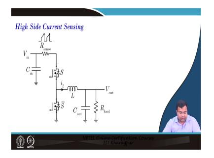
High side current sensing here if we consider then if we want to implement peak current mode control in analog it is possible, but if we want to implement digital peak current mode control can you use valley current?
