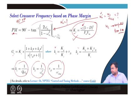
Now, how to design first you write the; that means, the select the crossover frequency based on the phase margin. So, if you set a desired phase margin to suppose I want to achieve let us say 45 degree is my desired phase value then you set this here to be 45 degree and solve this tan inverse, and there you will get what is by omega n value for the 45 degree phase margin.
