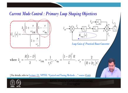
Now, if you take a boost converter, with the same current mode control only the topology got changed then we can write the loop transfer function for a boost converter if you write the control to output transfer function under current mode control we will get a right half plane zero and if we take an ideal boost converter we can drop this term and these are the expression it is given in Lecture 31 in our earlier NPTEL course.
