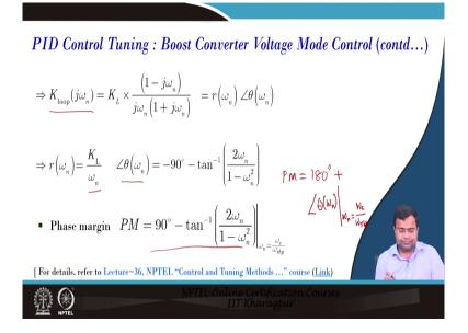
And this can be written in the polar form r and theta, which are this loop transform function, r is nothing, but K L by omega n. What is K L? If you write so, we have taken K L here this is the term we have taken K L; that means, K L is equal to F m which is the modulator gain of the voltage mode control; that means, the saw tooth. What is F m? We know F m is equal to 1 by V m. And what is V m? It is nothing, but the sawtooth voltage peak value is by V m peak value ok.
