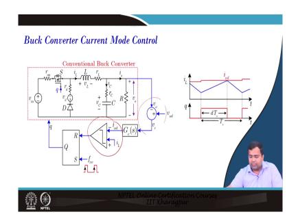
We know this is the implementation of current mode control, we have an inner current loop here and we have an outer voltage loop here and this is the peak current mode control.
