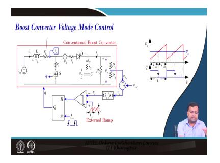
Now, we will be considering boost converter voltage mode control. So, again it is the same as the buck converter voltage mode control only the topology is different.
