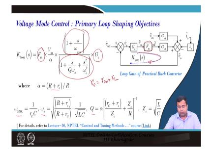
Now, if you go for digital voltage mode control what are our primary loop-shaping objectives? So, you can see this is our loop transfer function, loop yeah loop transfer function, then the loop transfer function is a product of the modulator gain and this modulator gain is coming for saw tooth waveform it is 1 by V m that is 1 by the peak voltage, then V in
