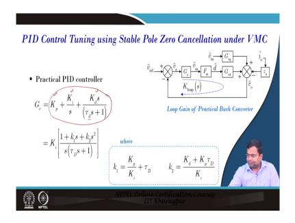
Then, we PID controller tuning for this voltage mode control we want to do for stable pole-zero cancellation. So, we can write a practical PID controller that we have discussed multiple times K p K I by s and K d this is a derivative filter time constant. Then, we can rewrite this equation in this form where k 1 and k t; that means if you simplify if you write the whole expression as a polynomial of numerator and denominator we can take K i out and these are the expression.
