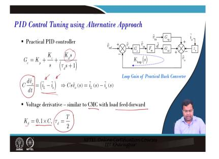
There can be an alternative approach to PID controller design because in digital control will mostly we are going to use digital PID control, which is why I am primarily focusing on PID controller, but in analog voltage mode control people use type - 3 compensators over PID controller.
