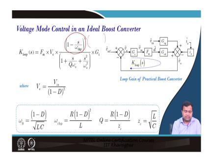
The same thing we can write the loop transfer function, the only here is that in the boost converter, we will have a right half plane 0. Here we are talking about the ideal boost converter in a practical boost converter we may also have an ESR 0. Since ESR 0 is far right-hand side so, it will be primarily dominated by the right-half plane 0. And what is V e?
