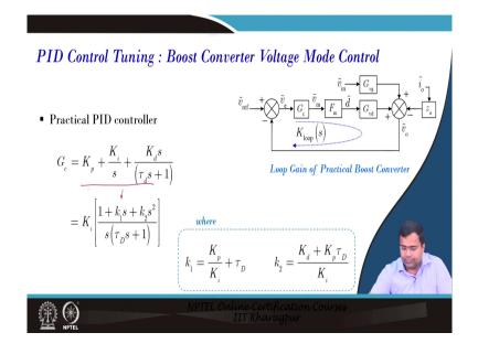
Now, if you take a PID controller in a boost converter how to design it? Again we write this PID, again you are initially going for exact stable pole-zero cancellation, again we are we can rearrange this PID into this form.
