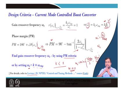
Then how to design? This is your r omega n and the gain crossover frequency r will be 1. So, you can get from here and this will give you crossover frequency is nothing, but k g into k c this is the system parameter. And once you; that means, this k c will be the controller here; that means, if you set omega c then you can find k c because this is unknown and this is known perfectly known.
