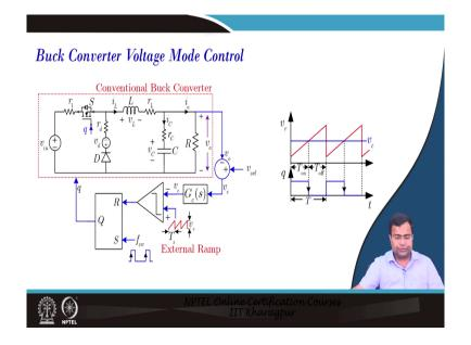
So, here we will first you know recall want to recall the voltage mode control buck converter we have discussed this you know diagram multiple times and you know this is a saw tooth waveform to generate the duty ratio.
