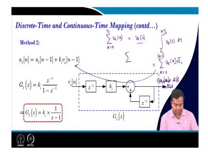
Now, by the same method if you go to the forward difference you see for the kth cycle; that means, what is the forward difference method for k equal to let us say 0 to T s, what is this in forward difference? It will be simply  $v \in 0$  we know that right, ok because it is only taking between 0 to T s this value.
