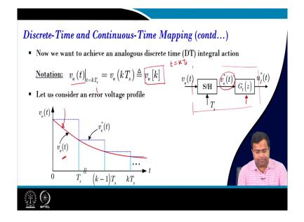
Now, to achieve an analogous discrete-time integral action first we have to draw the sample and hold. So, in digital control, this error voltage passes through a sample and hold circuit and this is the sample voltage error voltage.
