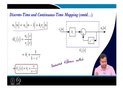
And then you can realize by inserting a unit delay and if you obtain the transfer function by this method you will get k i 1 by 1 minus z inverse. So, this is the integral transfer function in the z domain and this is using the backward difference formula backward difference method.
