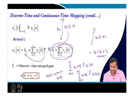
So, that is the iterative method sorry v e s sum; that means, let me write this integral once more. So, this is represented as v e s sum of this whole thing. Then, we can write k 1 to n minus 1 v e k as v s n minus 1. So, then by the iterative algorithm, we can write v e v s of n equal to v s of n minus 1 plus v e n that is it and this iterative method will be used to get this integral value ok. (Refer Slide Time: 12:23)
