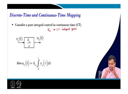
So, we will start with a pure integral control in continuous time and we are taking an error voltage v e t and it is passed through an integrated controller with an analog integral gain; that means, k ic which our continuous-time integral gain continuous-time integral gain and consistent of the pure integrator. And we can write the time domain expression u I of t k ic into 0 to t v e T. So, we are trying to integrate over time 0 to the current time.
