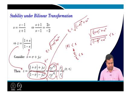
The next is under bilinear transformation if we write s equal to z minus 1 by z plus 1 and again if you simplify to write z in terms of s, now you write s equal to sigma plus j omega and you replace and you rearrange; that means, you obtain the z from here by substituting s in this expression then you will get 1 plus sigma plus j omega 1 minus sigma minus of j omega.
