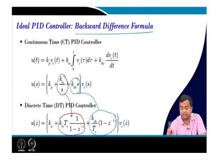
Now, we want to convert a PID controller from a continuous-time PID controller to a discrete-time. So, this is the continuous-time ideal PID controller parallel form and if we write in the Laplace domain it will be the function with 0 initial conditions. Then discrete domain if we use a backward difference formula what will be our integral gain? I mean we know that this term can be replaced by this term.
