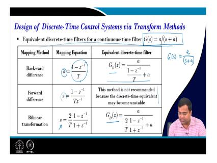
Now, design of the discrete-time. So, if you want to design then equivalent discrete-time for a continuous-time filter; that means,  $G \le 1$  by  $\le 1$  by = 1 by  $\le 1$  by  $\le 1$  by = 1 by  $\le 1$  by  $\le 1$
