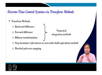
So, we will start with the discrete-time control system, if you want to design via the transform method what are the available methods? One is the backward difference, another is the forward difference, another is the bilinear transformation, then the step-invariance method, matched pole-zero and numerical.
