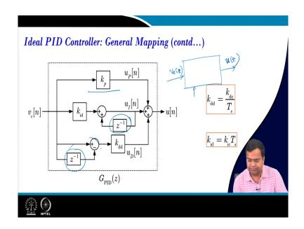
So, this is the formulation. So, if you want to realize this ideal PID controller so; that means, if your first term is straightforward it is simply going. In the second term, you have this one z in the delay term which is here in the feedback path and in the third term you need a delay and then subtraction. So, you need a delay this is delayed input and then a subtractor, multiplied by this digital derivative gain and this is the digital integral gain.
