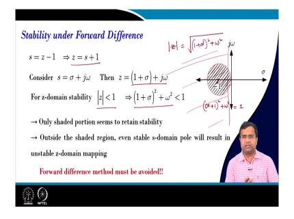
The forward difference we know is that z is equal to s plus 1, now if we replace s equal to sigma plus j omega then we will get z equal to 1 plus sigma plus j omega and we need to ensure that the z mod of z should be smaller than 1. And if you take the mod of this function what we will get? That means the mod of this z means will be the square root of 1 plus sigma whole square plus omega square, and the mod less than 1 means if you take the square it should be smaller than 1.
