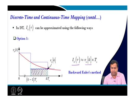
So, first method option 1, if we take this sample and then we using this sample we approximate; that means, it will be constant for this cycle for I mean as per this method we take this sample and then we take this area under the curve; that means, in this case, I k tau can be approximated to be v e k which is this sample value into T s and this method is known as Backward Euler method.
