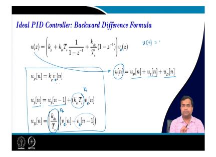
Then if you write this in the full form we can separate two things; that means if you take the inverse Laplace u of n, I want to write yeah it is written here which is the inverse Laplace of this it is coming from here. So, as if it is a PID controller it has three components, the component due to the proportional action, the component due to the integral action, and the component due to the derivative action.
