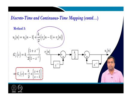
Next by the bilinear transformation, the only difference is the last term and here it will be replaced by the average of these two errors and which is written here if we obtain the implementation of this block and if you find the transfer function it will be k i by 2 z plus 1 by z minus 1.
