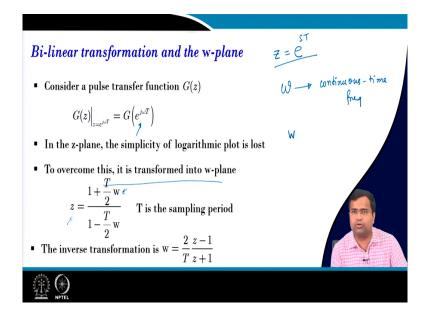
Now, this bi-linear transformation is when you get a z domain transformation; that means if you know that which is called pole-zero mapping it is z equal to e to the power S T. That is the exact mapping and that comes from the fundamental Laplace transform theorem; that means, if you go for you know how to obtain the transfer function using the Laplace transform and if you go to z transform by two basic theorem you can relate z equal to e to the power S T.
