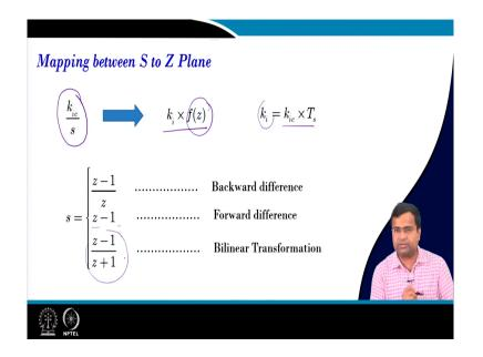
Now, if you want to map; that means, a continuous-time integration we started with and we got a discrete-time integration, and k i the discrete-time integral gain is this. What is f z; that means, if we map the S domain to the Z domain for the backward difference it will be z minus 1 by z for forward difference z minus 1, and for bilinear transformation is z minus 1 by z plus 1.
