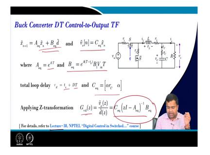
In NPTEL in this course; that means digital control in this particular course, in lecture number 31. Now, so buck converter discrete time control to output transfer function; that also we have discussed. Where we have obtained that the x n plus 1 tilde is equal to A equivalent to the x n tilde plus B equivalent to the d tilde and the output voltage is C equivalent to the x n tilde.
