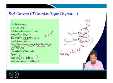
So, all these transfer functions we have plugged into the MATLAB model. W 0 practical then Q then after that e s r 0. So, the numerator, if we follow the transfer function, will be this denoted will be this G v d will be this, this is the continuous time, control to output transfer function without delay. And the delayed version of that will be the same transfer function, which means the polynomial numerator and denominator with an input delay which is t d.
