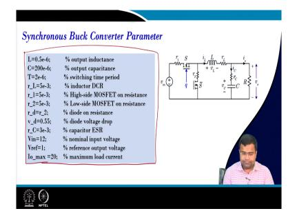
Now, we have considered the synchronous buck converter parameter, which is this and which we have considered for various other lectures. We have discussed also lecture number 35 and 36, where we have shown the large signal model validation. So, we have identified our discrete discrete-time accuracy, and it can exactly capture the cycle by cycle-by-cycle behavior with simulation.
