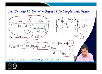
So, here if you remember our buck converter continuous time control to output transfer function; for the sample data system. So, we know G vd and this can be derived from our equivalent circuit model, this equivalent circuit. And we know in digital control there will be a total loop delay of t s plus DT. What is t s? That is the sampling plus you know computational time and DT is the DPWM delay.
