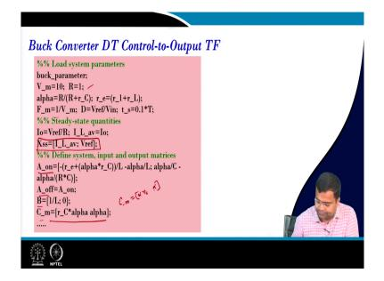
Next, where buck converter discrete time out control to output transfer function. Say again, the same parameter everything same V m, now we are using the discrete-time small signal model. So, for that, this will be derived around the steady state operating condition, and we are taking the average inductor current and the reference voltage. Next, we are taking on time matrix, off time matrix and, since r on rds, one's are identical for both the low side and high side.
