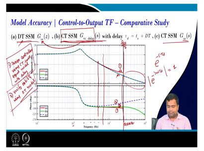
And this is the plot, in this plot, the first one is a which is this one, which is the discrete time control to the output transfer function, and since it is in discrete time, you cannot plot beyond half of the switching frequency. So, this is half of the because it is a Nyquist frequency range. After that it is invalid. Even for a continuous time also it is invalid because, we are applying an averaging technique followed by linearization, so it requires a minimum of 2 cycles to get the effect.
