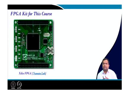
So, the FPGA kit that will be used here is a Spartan 6 FPGA we are going to use, but yeah one can use any other FPGA.
