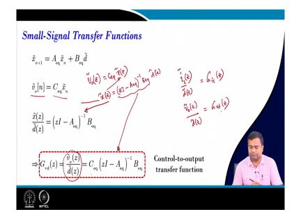
Next, we want to derive control of the output transfer function. So, v 0 n is already a function of x n; that means if we apply the Z transform; that means, we can get v 0 z as a function of C equivalent to x z. And what is x z? We know the x z tilde is equal to z I minus A equivalent inverse B equivalent into d hat z and this is exactly shown here. Then, if we substitute this into this equation we can get this equation.
