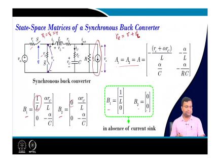
Now, if we take the synchronous buck converter and since we are considering this r 1 and r 2 are equal because we have taken r 1 is equal to r 2 equal to r and where r e we have taken r plus r on that is sorry r L that is the DCR of the inductor. Then, we can write all A matrices are common; B 1 matrix will be 1 by L term will be there for B 2, it will be 0. If the load sink is not there if we remove this path then B 1, and B 2 will be simple like this. So, B 2 is a null matrix.
