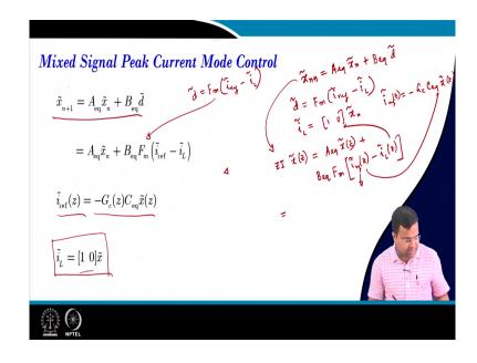
So, we can write this out. Let me write this term below. So, it is B equivalent to F m. Now, what is i ref z? i ref z is minus G c into C equivalent into x z. So, if you write Z domain. So, this is z; which means. So, here it will be what? i ref z minus i L z. So, what is i L z? That means, this you replace with this, and this you replace with this.
