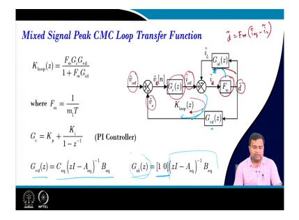
So; that means, this is the loop transfer function under peak current mode control. You see this is the reference voltage minus the current voltage output voltage. This is the error voltage that goes to the controller. It generates the reference current level, then this reference current level minus i L is nothing but your error current. And, if you multiply with the modulator gain it will generate the duty ratio because we know that the duty ratio is nothing but F m i ref minus i L.
