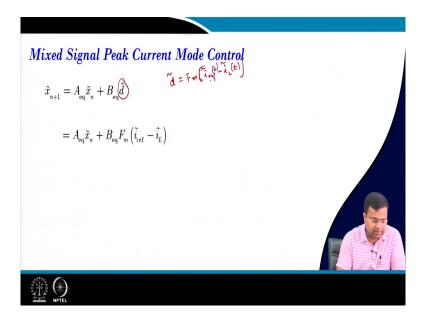
Now, we start with this. So, we replace the duty ratio, what is the duty ratio we know? The duty ratio is the modulator gain then I ref perturbation minus i L perturbation.
