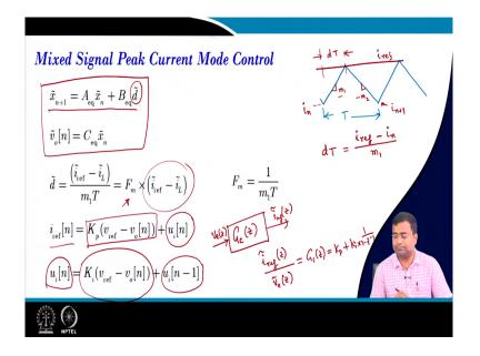
Similarly, if you take the mixed signal peak current mode control we can start with the very fundamental equation which is the perturbed model, but in current mode, the difference is that the generation of the duty ratio is different. In voltage mode, the duty ratio is generated from you know, how it is generated? If you take a controller the output of the controller is compared with the sawtooth waveform and that generates the duty ratio.
