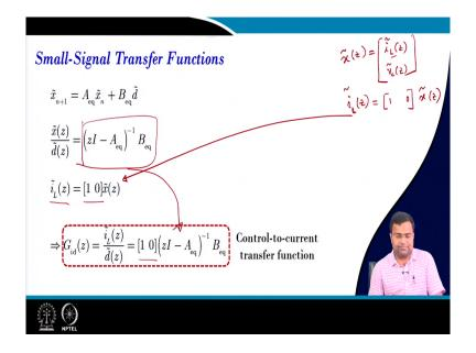
That means if we want to get the current too. So, how to extract current from the x z? You simply multiply with 1, 0 matrix, then it will give you the first term because we know what is my x z tilde. It is nothing but i L z tilde and this is the v c s z tilde where v c is the capacitor voltage. So, if we want to take the first element; that means, my i L z tilde is equal to I will simply multiply with this matrix into x z.
