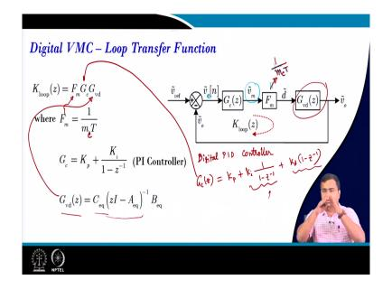
Now, we will show if we draw the block diagram. So, this is our error voltage, then this error voltage goes to the controller, the controller will generate the modulating signal, and then it goes to the duty ratio. So, here this F m is nothing but 1 by m c T ok. So, if you use a different color it is 1 by m c into T. This is our Fm. Then, we have already derived the v 0 to d transfer function in the z domain and that itself takes care of the delay and all.
