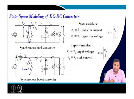
So, if you recall you know the state space modeling of a DC-DC converter if you take a synchronous buck converter with practical parasitic and we can also consider a synchronous boost converter. So, where we can consider the inductor current and the capacitor voltage as the state variable and we can also take the input variable as the input voltage and the load current if we consider an additional sinking load.
