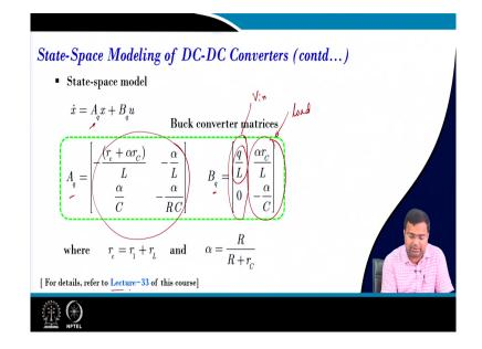
Next, if you want to write the state space model then based on the switch configuration whether the q is the gate signal whether q is 1 or 0, we will get accordingly A 0 or A 1. And
