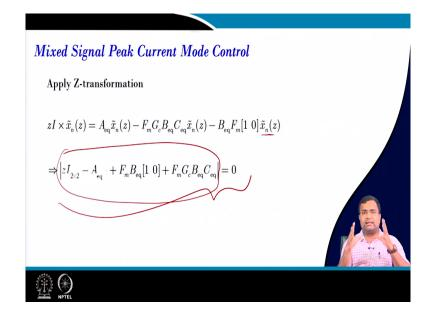
And after that, you will get the overall characteristic equation. And you can take everything on the left side because x z can be taken commonly. So, we will get the characteristic polynomial like this. And this equation is the characteristic equation. So, from here we can find out the eigenvalues to check whether all are inside the unit circle or not.
