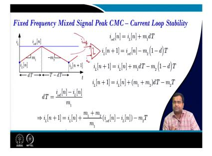
Remember, in mixed-signal current mode control your reference current and the inductor current are in analog. So, one can expect for the same reference current the mixed signal inner loop stability; that means, the zero input stability must be identical because they are identical in terms of the analog current loop. So, only the digital part will come here when the mixed signal will have a digital compensator followed by a D to A converter that we have seen.
