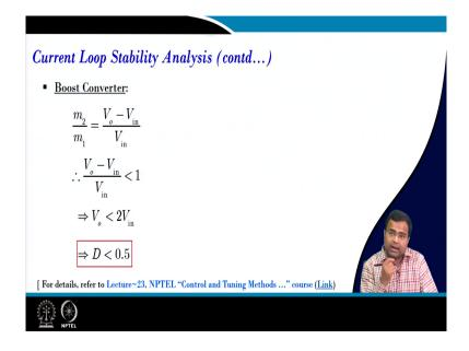
Similarly, for the boost converter if you take again m 2 by m 1, and if you get V 0 by V in that term because if you take mod of m 2 m 1 since both are positive. So, it will be m 2 by m 1 should be smaller than 1, because it is always greater than 0. Then, again it can be shown the duty ratio should be less than 0.5. So, it is a universal requirement the duty ratio should be smaller than 0.5 with a closed inner loop.
