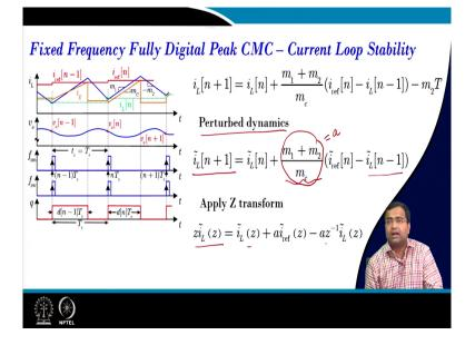
So, this is the one, now I want to again do the perturbation because I want to do perturbation and I want to see the effect. So, here if we perturb the initial condition we can find out what is the requirement of the stability of the i ref n is constant. So, now if we apply the Z transform here then, since it is a perturb term there is an initial condition is for this term; if you straightway apply the perturbation it will be z into i l z then i l z then this I have taken a.
