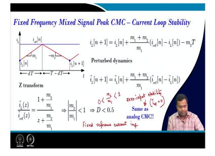
And, you can show you know subsequent perturbation that if you take the z transform it turns out again mod m 2 by m 1 should be smaller than 1. And since m 2 by m 1 m m 2 and m 1, both are positive. So, you require that m 2 by m 1 must be greater than 0 which is true and it must be less than unity; and again it will come to less than 0.5. So, I do not know going through all the steps because we have already discussed the analog current loop.
