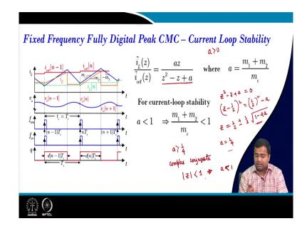
So, you are interested here. And that can be proved that it will be true if we take a less than 1. It can be easily proved because if I write z square minus z plus a that equal to 0, I can write z minus half whole square is equal to 1 by 2 square minus a. So, I can write z equal to 1 by 2 plus minus; if I take half common what we will get? We will get so 1 minus 4a, correct? So, now, you can see a is always greater than 1.
