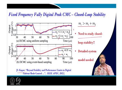
But once you close the outer loop I am just showing an example because I will go to this closed loop analysis later. So, here I am showing if I just close the outer loop and if I set m c equal to 1.1 times because this is greater than; that means, I have taken m c to be greater than m 1 plus m 2. But, with the closed loop you see the blue lines indicate there is subharmonic oscillation.
