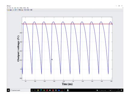
Interestingly, you will find, since you are sampling here, that means, we are sampling whenever the inductor can hit the peak current. That means we are almost sampling at the peak voltage.
