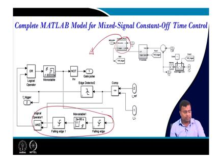
And if you go inside the constant off-time modulator then you will see this block. So, this block takes I ref and I L. So, whenever the inductor current hit the peak current, the rising edge comes and that will trigger the monoshot timer. And this is the additional block that is used to minimum off-time, and minimum on-time because it requires a minimum on-time.
