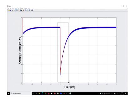
So, now, this shows the load transient, the load step of the transient case study.
