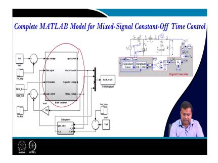
And this is a complete block diagram, we are going to MATLAB. So, this is the power state that we know and this is the controller.
