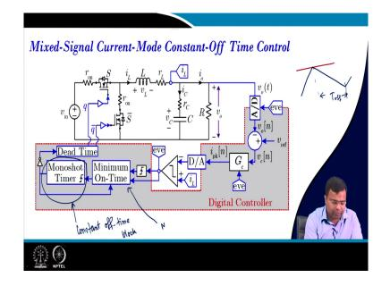
So, if you talk about mixed signal current mode control constant off-time control is analogous to peak current mode control. And we know that if we take any peak current mode control here, so in this particular case the current will rise and then fall like this. So, here our off-time is fixed. So, off-time is fixed. So, that is why it is analogous to peak current mode control. The only difference here it is a variable time control where the off-time is constant, but the time period can vary.
