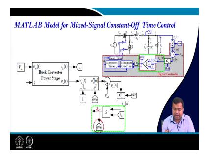
And that means we have this event created from this comparator output when it is just triggered and this rising trigger actually will generate them, enabling the monoshot timer because you have to turn on the constant off-time block.
