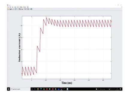
So, where if you go to the inductor current, the inductor current is changing from you know initially it was 1 ampere average current, now it is changing to 21. So, a 20 ampere load step size, ok. So, this is the output voltage response. It is a sluggish response, but we have not discussed about the compensator design. So, what I am saying here? Here we have considered T by 100 as the minimum on-time, but you can customize it. So, you can customize the other parameter.
