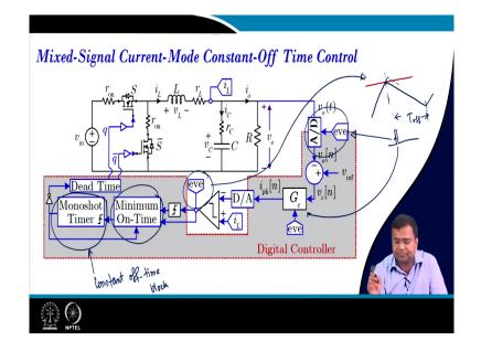
So, this block is the minimum on-time. Then, the same we need an A-to-D converter which should be sampled using an event clock. So, here event again is a comparator. So, what is the event? Here the event is this is the event; that means, whenever the inductor current hit the peak current that is the event. But in the practical circuit, even if it hit the inductor current will hit, the peak current may turn off a little later because there will be some delay due to the comparator, and driver.
