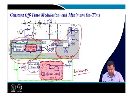
We have discussed the 23 also, we have discussed 23 as well where we have compared various things. So, this is in our past lecture on control and tuning method in switch mode power converters. So, all these blocks are common. This block is common for analog control as well as this mixed signal control, but this block is different up; that means, this block is different including this DAC. Remaining this analog comparator everything else is common.
