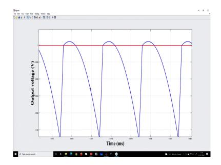
So, that is why your peak voltage is regulated at 1 volt, but not the average voltage. So, to solve this regulation problem, we may have to shift the clock edge a little bit. That means if we take to let us say we sample somewhere in between; that means because during this time your switch will remain off and when the switch remains off; that means, your monoshot
