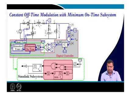
So, here as I said this is common and I will go to the MATLAB Simulink block, and we have to incorporate the minimum time.
