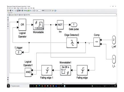
So, if we go to MATLAB. So, let us go to MATLAB. So, this is the complete representation of this circuit, buck converter, and whatever we have discussed. And the trigger pulse is generated from here; that means if you go to this monoshot timer sorry; the comparator
