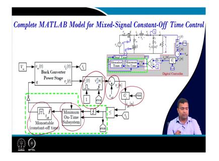
Then, we will go for custom the complete MATLAB model. You know this will be the event trigger ADC, error voltage, then controller, event trigger compensator using difference equation, minimum on-time, and then this is the constant off-time modulator.
