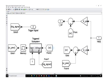
So, this is a PI controller. And we have discussed this block. The same as constant on-time as well as fixed frequency control. Only the clock is different here. We are using a different clock. And here we are using non-uniform sampling or event base sampling. So, it is different from the uniform sampling. Next; that means, we can realize the PI controller using a difference equation and using a clock-triggered operation.
