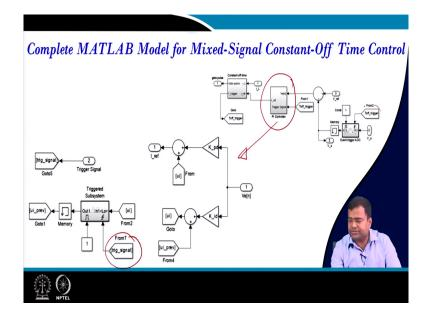
And if you explore this block, this block we have discussed multiple times, the only difference is the trigger pulse is different here. That means, we are using this trigger pulse and this is created from the comparator output.
