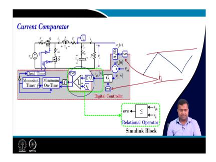
And that will be compared with the actual sense inductor current and that is the comparator that is in the analog domain that we have discussed. Whenever it hit the peak current; means, whenever the inductor current hit the peak current; that means if you draw the peak current reference and that is the point we are taking this event. So, this event is passed through this. It is generated, ok.
