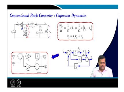
And the conventional buck converter. If you take the capacitor dynamics then the capacitor voltage capacitor dynamic output capacitor dynamics d v c it can be written like this and this
