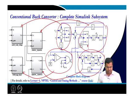
So, the complete conventional buck converter, you can get this detail in this NPTEL online from our previous lecture in lecture number 4. So, here we are not again wasting time to again you know explain the all details of the power stage architecture, but this represents the complete block diagram of this converter.
