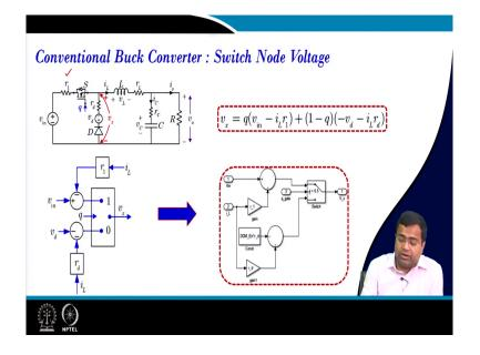
How does it realize? That means, if you take the switch mode voltage it is q v in minus I L r 1 r 1 is this one, then 1 minus q minus v d I L r d. So, v d is the direct voltage drop r d is the direct resistance drop. And this can be implemented using this logic and we can create a DCM that enables logic like this.
