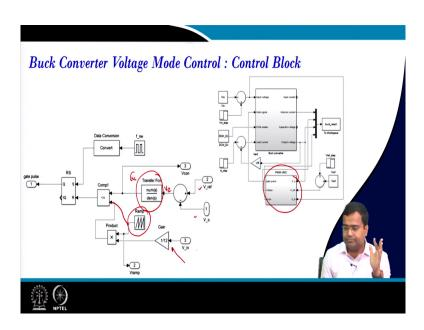
In this diagram what is inside? Inside this controller; that means, you are taking the reference voltage and the output voltage and this is the error voltage this is the controller which is GC and we will program this GC from outside; that means, the transfer function will be the poles and zero that will program from the outside right or you can realize inside also there is no
