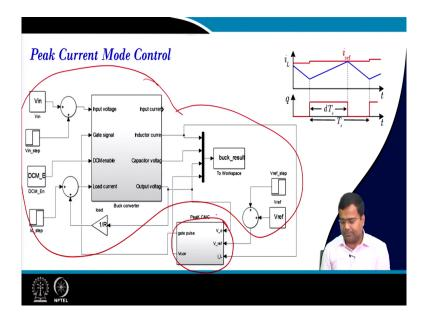
Then in this course in this class, I will also show the MATLAB simulation of peak current mode control. What does it look like? So, peak current mode control means your reference current inductor current is compared with the reference current. This is a complete block diagram you see this block remains the same. So, overall this block remains the same we are not touching this block, but only this is going to change ok.
