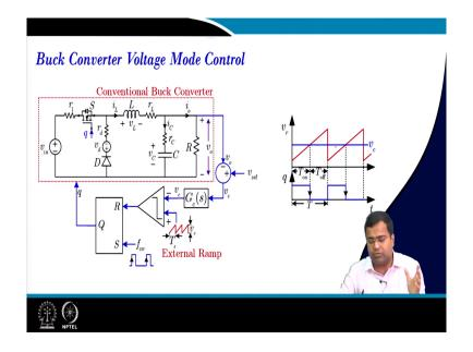
So, first, we will take the buck converter voltage mode control. So, here this is a conventional buck converter. It can be a synchronous buck converter also and we are talking about a voltage mode controller we know about the sawtooth waveform and the control voltage is compared to the sawtooth waveform to generate the acceleration.
