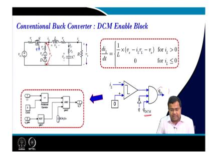
So, this DCM enables block; which means, we have a DCM enable if we set it to 1, then it will enable this DCM block depending upon whether the inductor current is touching 0 or not. But, if you set it to 0, then it will not the inductor current can go to in the negative direction. Because this always will be 0; that means, the DCM enable logic is a DCM enable logic is disabled and this is the overall block diagram for the DCM enable logic.
