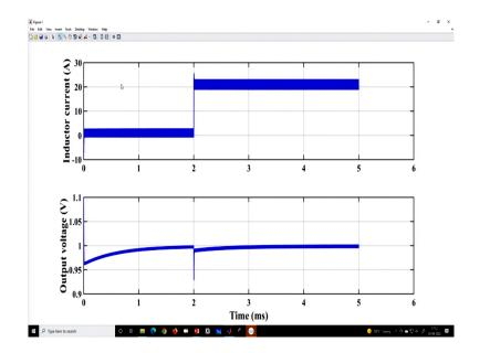
And this is the load transient performance. You can see this is the inductor current and this one is the output voltage.
