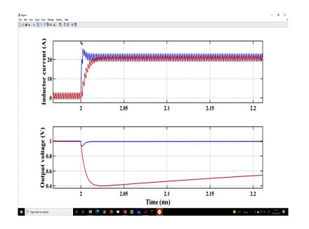
So, because we are using an adapted value of pi value. So, if we increase the proportional gain we can speed up the transient performance, but generally current mode control we saw in our earlier course that the current mode control behaves like a first-order system. So, that is why it is kind of an overdamped response. So, unless you do load current feedforward it will be somewhat difficult to speed up very fast within the small signal control bandwidth.
