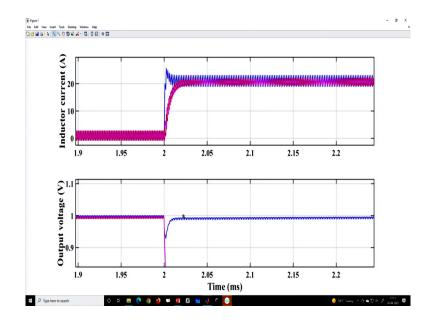
I am talking about red and magenta. They are more or less the same, but the voltage mode control is different because we are using a PID controller and we have discussed earlier that this derivative action is set in such a way it will look like you are providing sufficient damping.
