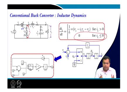
Similarly, if you go to inductor current dynamics, we can write di L at 1 by L, and this particular term is incorporated to enable the DCM operation it can be realized by this and you can get the complete block diagram using this architecture.
