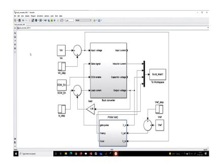
So, let me go to MATLAB. Now, this is the MATLAB block diagram of this voltage mode feedback control of a buck converter. Here this is the power stage; which means, the power converter.
