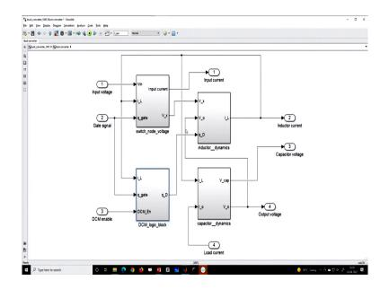
And you know if you go inside, then the switch mode voltage inductor current dynamics the DCM enables logic then the capacitor dynamics. And this accepts the input voltage where we can also apply a step input voltage here is the DCM enable logic if it is set to 1 it will become a conventional buck converter. If it is 0, it will become a synchronous buck converter. Then
