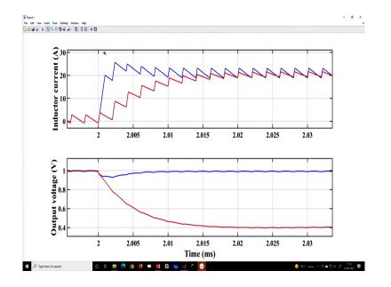
So, you can see the current mode control we have not tuned properly, but it is only a pi controller not sufficiently high gain. So, that is why the response is much more sluggish ok.
