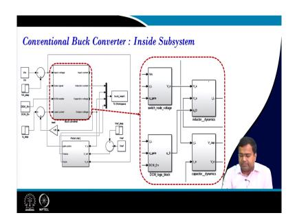
Next, if you go inside this converter. In the power stage, I have shown you the switch node configuration then inductor dynamics DCM logic, and capacitor dynamics.
