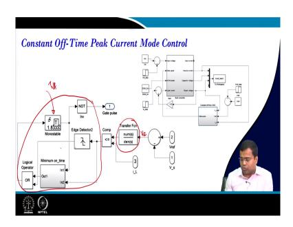
How does it operate? Here again, it is the error voltage, it is the compressor. So, this part is common, and here is the inductor current. But, after this comparator this whole logic is different. In fixed frequency, we had a latch circuit, but now instead of a latch we have a mono short timer and this is loaded with the constant of time ok.
