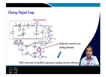
Now, when you close the digital loop, then this inductor is in analog and this is in digital. So, you cannot use a mixed domain thing directly. So, you need to have a D to A converter and which we have also discussed in the previous class.
