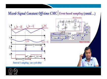
So, in constant on-time off-time this is with one cycle delay; that means, you can provide sufficient delay for the conversion and computation ok.
