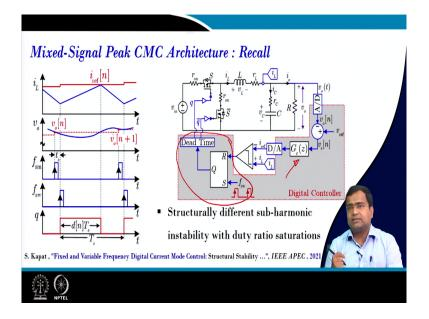
So, in this lecture first, we will talk about mixed-signal peak current mode control architecture. If we talk about if you recall the fixed frequency control then we know here only the difference will be the modulator. So, this modulator will be different otherwise you know you have an analog comparator then you have an A to D converter and D to A converter.
