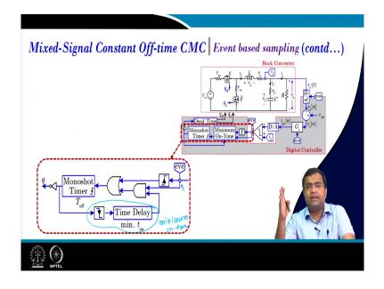
So, this is a full architecture, and the monoshot timer has a detailed description; that means, you know if you go inside the monoshot timer there will be a time delay and this delay is a minimum on-time. So, this is our minimum on-time, if we want to avoid a complete collapse of the system minimum on-time and this is there in all commercial products and if you talk about constant on-time there will be minimum off-time.
