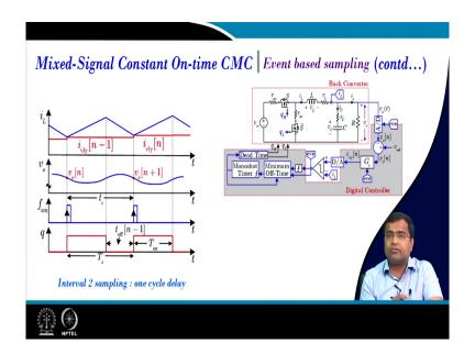
So, this is the constant on-time current waveform here you can see if we take thus it is one cycle delay. That means if you take the sample whenever the monoshot timer is about to turn on; that means, you know this again will be delayed. That means, whenever the monoshot timer the current hit the reference current limit then actually you send them because it is one cycle delay.
