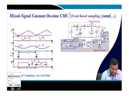
So, if we take them here. So, it should be the current should go a little bit on this side, and then it will have because this is the time the dead time a delay due to the driver as well as the dead time. So, that time you can take the sample and you can use it in the next cycle. So, it's a one-cycle delay. So, otherwise, it is the same only fundamentally how this modulation and the timings parameters are generated that is the difference.
