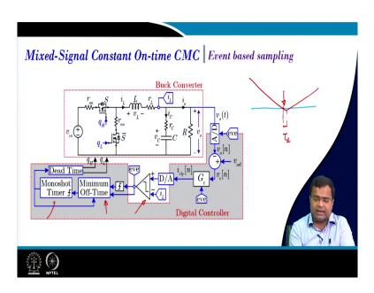
And this will also have a potential problem in terms of stability and performance if you go to constant on-time. So, this architecture also we have discussed here is like a valley current mode control; that means when the inductor hit the lower limit current. That means, whenever the inductor hit the lower limit than you turn off the; that means, you should send
