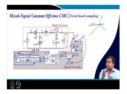
Then if I take the full structure of the constant off-time control, we need to compute this A to D coA-to-Dr. That means, we need to sample the voltage of like A to D converter using the A to D converter that sampling should be with responsering. So, when you say the event this is a clock that will generate the event and that will sample the A to D converter. The same clock should be used to sync with the controller computation ok.
