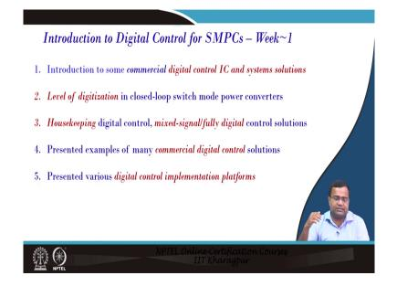
So, now we want to summarize weekly basis. In week 1 we introduced the digital control in the switch mode power converter. We have introduced some commercial digital control IC, IC, and system solutions, and we have discussed the level of digitization in closed-loop switch mode power converters.
