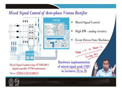
So, this is another one from ST microelectronics the 3-phase Vienna rectifier where it is a mixed signal control, and the inside of all these control logics are not available, but it said that the event-driven state machine is using a mixed signal control.
