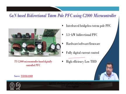
Another aspect is a GaN-based totem pole you know PFC interleave PFC which is like a using C2000 microcontroller. This architecture was considered with a small hardware demonstration in this course in week 9.
