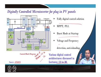
So, then solar microinverter in plug-in PV is for micro ST microelectronics where it also uses you know fully digital control solution and burst mode control for light load efficiency improvement and we have discussed various digital control architecture in lectures 11 12 to 20 and we have also discussed in week 10 week 8 and week 10 to 12.
