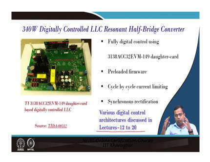
Then digitally control resonant half-bridge converter this is from you know Texas instrument which also uses the fully digital control solution. And we have discussed various architectures of digital control from lectures 12 to 20. So, some of this architecture including extensive implementation from week 8 as well as weeks 10 to 12 will be helpful.
