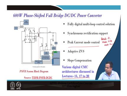
Then this is a phase-shifted full bridge converter from Texas instrument which also uses fully digital control multi-loop and again we have discussed multi-loop digital control both fixed frequency variable frequency as well as keep peak current mode control. We implemented this thing in week 8 then from week 10 to week 12 different architecture.
