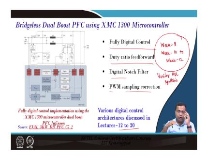
Then we are talking about a bridgeless dual boost PFC and this is for Infineon technology, where you know it talks about high power density 3 kilowatt PFC, and it takes it to consider fully digital control and which has a duty ratio feed-forward notch filter and sampling, but all details of this control architecture may not be publicly available.
