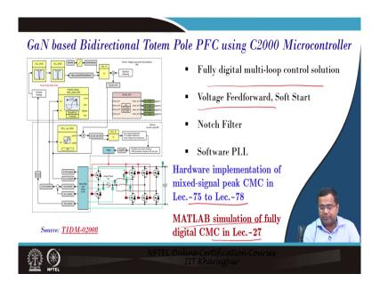
And in this course, it is a 3.3-kilowatt converter and it is fully digital current control the other feature of this controller it uses a fully digital multi-loop control solution and it also has a feed-forward soft start. Now if we recall our digital current mode control architecture we
