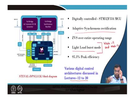
Then this is the 3 kilowatt LLC converter from ST microelectronics, then it uses you know fully digital control solution and adaptive synchronous rectification; that means, you can also do you know burst I mean the dead time optimization.
