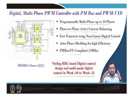
Next, if you go for this ampere solution where we are talking about intelligent phases and the whole loop in the digital controller in digital. So, you can hear it is offering multi-phase for scalable phase up to 10 phase to phase active current balancing then fast transient digital control.
