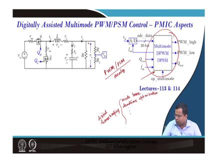
Then digitally assisted multi-mode, so we have discussed multi-mode where we are switching between PWM and PSM. So, this can be easily implemented in analog because there is a commercial product available where it does not require any digital. So, it can be implemented in analog control very effectively, but we have discussed the mode transition effect and then dead time optimization. So, mode transition then dead time optimization during dead time optimization.
