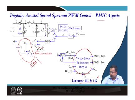
Then if we go for space spread spectrum modulation we discussed with bi frequency DPWM in lectures 111 and 112. Even if you keep everything in the analog loop you can only adjust this person and link with your sawtooth. So, that you can have a bi-frequency operation, you do not touch the loop compensator anything because we show in lecture number 112 and 11 112 experimental results that the performance has no effect.
