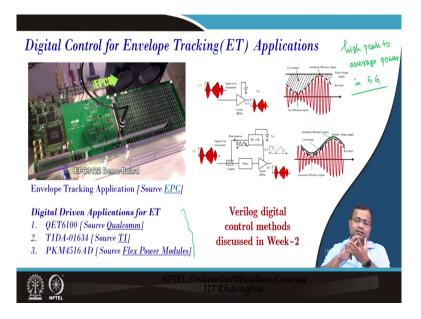
Then there is another application for envelope tracking where if we are talking about 5G communication you know then adders we need a very high-speed power supply for envelope tracking, where the envelopes will change drastically and particularly you can have a very high peak to power high peak to average power in 5G.
