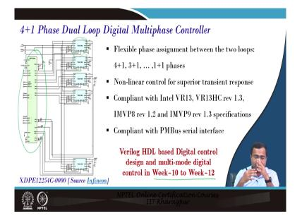
Then this is another Infinium where the flexible phase is also a digital control solution where you know again it is a multi-phase you can have a non-linear controller for very fast transient all this can be possible in the digital domain, but we are not touching the power stage which is in analog.
