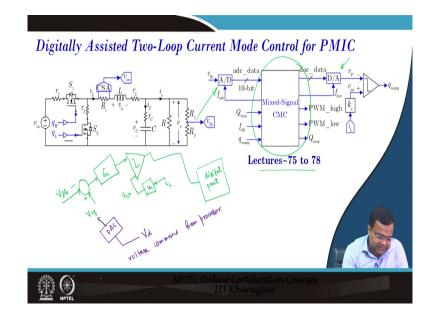
So, that means, the cost of the silicon area of these things matters. Now we are going to two loop control current mode. In lecture number 75 to 78, we discussed the mixed signal current mode control. There we need an A-to-D converter and we need a D-to-A converter. Now, this may not be affordable for many applications because your ADC cost may be high power consumption the delay can be high and that also may be expensive.
