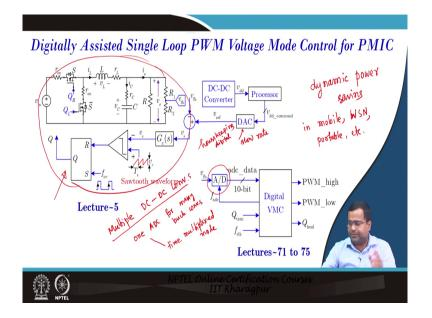
If we start with our digital voltage mode control that we have discussed in lectures 71 to 75, now how can we make a high-frequency digital control voltage mode control power management IC where the power is constant? We cannot afford to have let us say adc; that means, it will be expensive or it can be power hungry the silicon area can increase, but we still need to support it.
