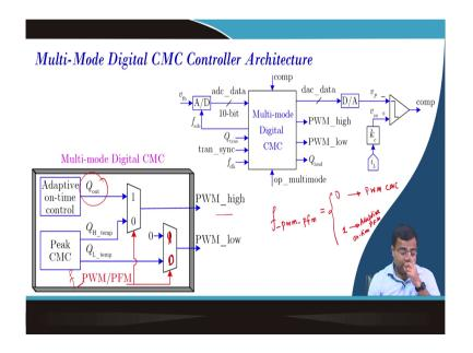
Now, this is the overall block and if we recall the earlier lecture I mean lecture number 114. We wanted to integrate that PWM and there we did PWM PSM here PWM PFM. So, the methodology of selecting the high-side and the low-side gate signal is the same; which means, it can take directly the adaptive on-time output.
