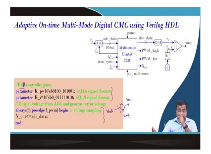
Then we need only the PI controller, not the PID controller PI controller gain. Because current mode control uses a PI controller this is for voltage sampling. Because we are sampling this voltage for the fixed frequency control where this will generate I N out and this n out will be subtracted from your N ref to generate an N error this error will go to the PI controller.
