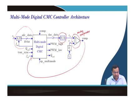
Now, we want to discuss; that means, we know for any current base architecture for digital we need a DAC and DAC will generate the current reference, and that current reference is the current analog comparator. This is our analog comparator, analog comparator and this comparator output is coming here.
