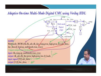
But now we want to develop this multi-mode control. So, this is the main module again I want to link; that means, this is your ADC data; that means, let us have ADC data. So, this ADC data is coming here ok. Then f the clock is here ok Q then we are generating inside, so this is you are here. Then we are also giving another option for this multimode trans sync we are giving here. We will see what is this is an external switch you know then the high side gate signal which is here.
