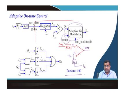
We have also discussed adaptive on time where the same thing this data to this adaptive on time modulator and we after that adaptive on time this is the comparator output; that means, here also which is not shown here there will be DAC. So, it is like an I ref current reference it
