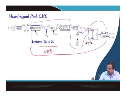
Now, we have discussed the mixed signal peak current mode control in lectures 75 to 78 in sufficient detail that how to use a register then this part will be your inside the FPGA. Then this part will also come and this whole part will be inside the FPGA that we have discussed.
