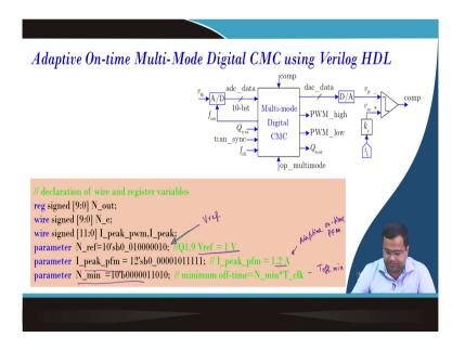
Now, we are defining this I ref this is linked with the V ref reference voltage. So, this is linked with the V ref equal to 1 parameter peak current limit. We are setting the pfm 1 for adaptive on-time pfm and this is the minimum this corresponds to the cut-off minimum because any on-time modulator should have a minimum of time.
