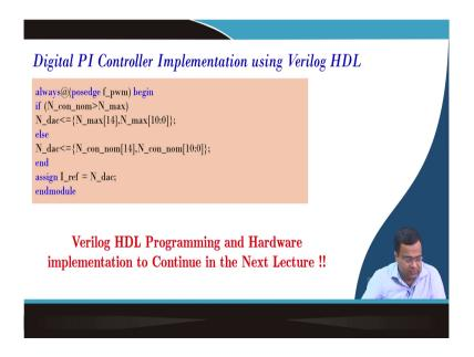
So; that means, we are making an integral reset when the PWM control is not activated that is the PI controller. Now we are going to continue this Verilog code for the other block in the next lecture that is it for today.
