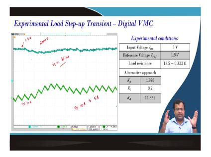
Now, here we are considering 5 volt and 1.8 volt where the load step again load resistance remains the same. But now there is a step up transient from 70 milli ampere because it is a 5
