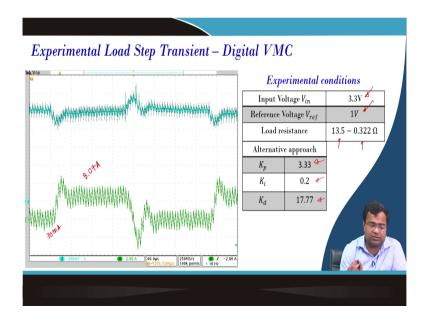
Now, we are first considering a first case study of load step transient where 3.3 volt input and 1 volt output and the load resistance is changing from 13.5 to 0.322 ohm and back because this is step up and step down. And we are designing using an alternative approach K p and K d are coming from the design which we made in the previous lecture only you have reduced K i and limited it to 0.2.
