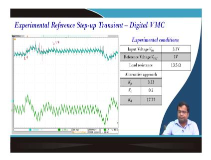
Now, we are talking about reference step up transient the reference step up transient if we take the zoomed version of this. So, this is the reference step-up transient in the average sense. So, there is an additional overshoot of around 50 milli volt and it is changing from 1 volt to 1.1 volt and this is happening as you know like an around 25, 30 microsecond.
