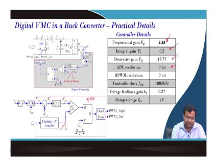
And initially, we are considering you know the 3.3 volt input and this is the design parameter for 3.3 volt input which we have discussed in the previous lecture which was considered the simulation case study derivative gain. Only we have reduced the integral gain because you know otherwise in hardware there are some other un-modeled dynamics and delays.
