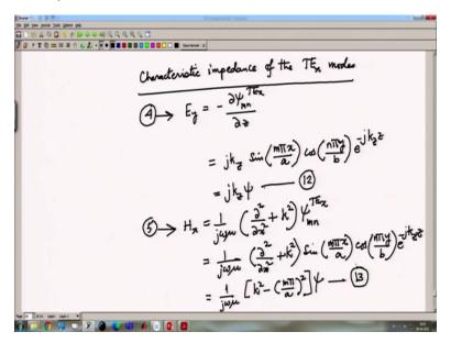
Then for the characteristic impedances of the TE to x modes we obtained from equation 4, Ey equal to minus del psi mn TE to x del z that is equal to j kz, sin(m pi x/a) cos(n pi y/b) exponential to the power minus j kz z that is equal to j kz psi. This is equation 12.
