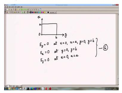
Now, for the rectangular waveguide, which is given here, the boundary conditions on the problem would mean, that the tangential components of the electric field will vanish at the conducting walls that means Ez must be equal to 0 at x equal to 0, x equal to a, y equal to 0, and y equal to b. Similarly, Ex must be 0 at y equal to 0, and y equal to b, and Ey must be 0 at x equal to 0, and x equal to a.
