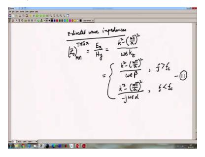
So, therefore, the z directed wave impedances are (Z0)mn for the TM to x mode as Ex by Hy, that is k square minus m pi by a whole square divided by omega epsilon kz and that is equal to k
