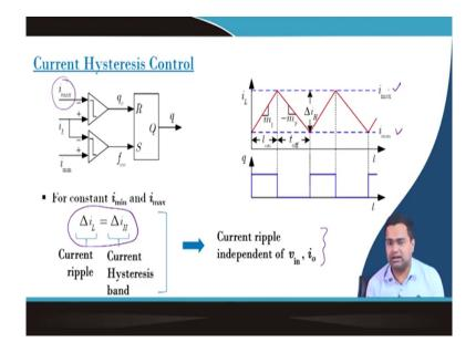
So, Current Hysteresis Control we can consider inductor current and again we can keep the inductor current between the upper and lower value the maximum and the minimum value. And we can now, if we use a fixed current reference like an upper and lower than the hysteresis band, the inductor current ripple can be made equal to current hysteresis band.
