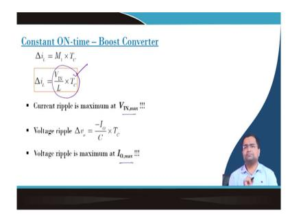
And if we take the Boost Converter current ripple expression, it can be computed that rising slope into on time. Since on time is constant, then you can see the current ripple for a given on time is maximum when the input voltage is maximum.
