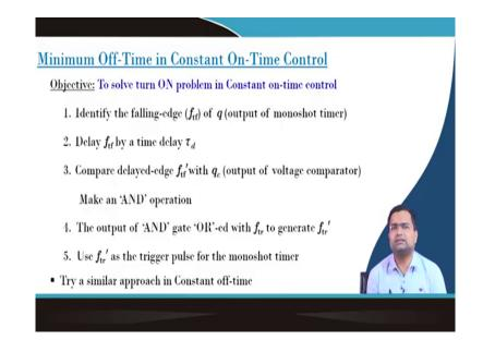
So that means, we can solve the problem of minimum off time in constant on time control problem. Now, minimum off time in constant on time control, how to summarize like what are the algorithm, the first we need to solve the turn on problem in constant on time control and this is particularly the case when after the switch is turned off.
