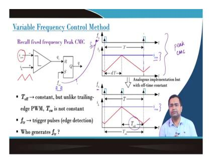
So, variable frequency control method I mean you know when you say variable frequency, because in the previous lecture we found that on time off time and total time. In pulse width modulation, we kept total time constant and we varied on time or off time like you know we saw in the previous lecture, like whether it is a trailing edge or leading edge modulation.
