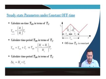
Again if we derive the Steady state Parameter under Constant OFF time control, since we have derived all this steady state parameter in my earlier lecture using timing parameter on time off time. So, you have to just replace this parameter and find out you know what are the like you know inductor current ripple, what is the inductor current ripple expression output voltage ripple expression and so on.
