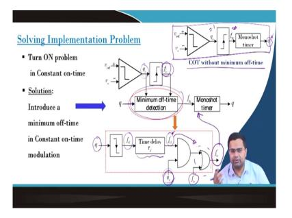
So, how to avoid such scenario how to solve? That means, in because in commercial constant on time controller you need to put. So, this is a straightforward that we discuss. It is in the very basic form now the turn on problem. That means we need to turn on the switch if we find that the output voltage is lower than the reference voltage, otherwise the voltage cannot rise. So, how to solve this problem?
