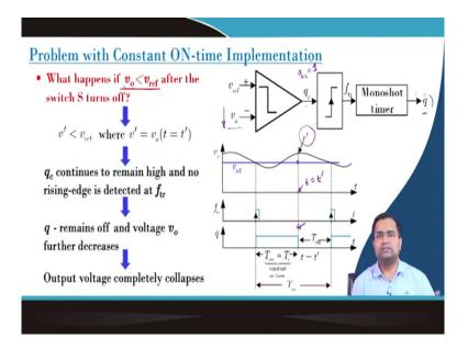
So, what is the problem with the constant on time modulation? Now we assume that when the switch turns off, that means I am talking about this phase when the voltage is v dash we are assuming the output voltage should be above the reference voltage and this is typically happened for steady state condition if you have sufficiently higher on time.
