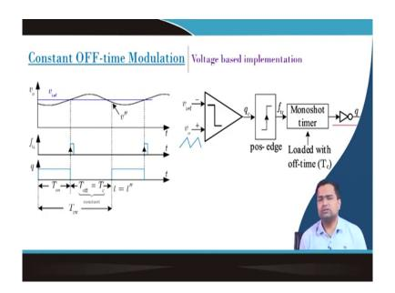
So, both techniques directly control the peak current. Now we can implement this constant off time using voltage based also, in this case we need to compare the output voltage with the reference voltage the same way and then the comparator output we are putting a like a positive edge detection circuit and then there is a monoshot timer and then again this is an inverted signal.
