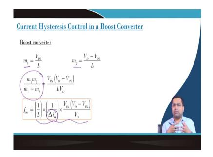
Under current hysteresis control for a boost converter, we know the rising slope, we know the falling slope and in our original expression we need to find out this m 1 m 2 by m 1 plus m 2. If you substitute then you can get the switching frequency which is again a function of input output voltage, hysteresis current and the inductance value.
