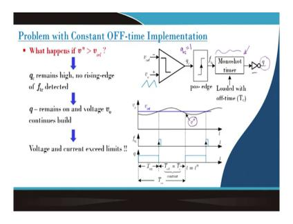
Again similar to constant on time, constant off time also have a problem of off time problem. That means, what is the logic here let us consider this v double dash and suppose we want that means when the switch is on we want that the output voltage should be lower than the reference voltage.
