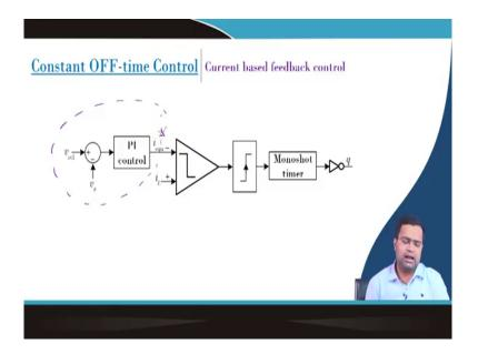
So, you can face a similar problem; that means, the current base constant off time control. Now, if we want to do closed loop control, then we can use a PI controller using the current loop that we will discuss in current mode control separately. But earlier we are using a fixed constant like a peak current, but now we can generate that peak current from the closed loop.
