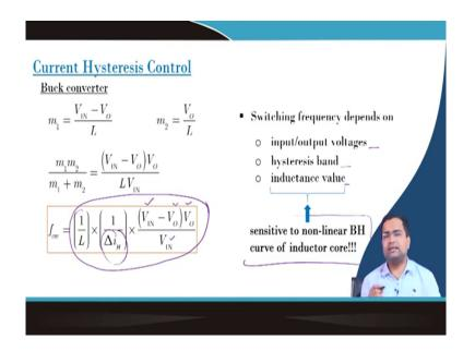
And for a buck converter, if we replace the rising slope and falling slope, then the switching frequency can be shown to be a function of the current hysteresis band, input voltage, output voltage as well as the inductance value.
