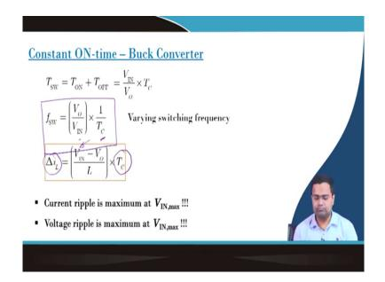
So, if we want to derive the inductor current ripple; that means, if we just the switching frequency can be derived from the voltage gain and it can be shown that under constant on time control the switching frequency is a function of voltage gain into 1 by T ON. So, if the on time is kept constant for varying input voltage switching frequency varies. If we take the
