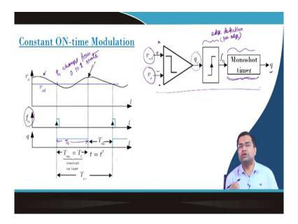
So, we want to first consider constant ON time modulation. What does it mean? If we take the output voltage of it can be a buck or a boost converter or any DC DC converter. If we compare this output voltage with the reference voltage and this is a comparator. And what does the polarity shows? This is a comparator and output of the comparator is a q c.
