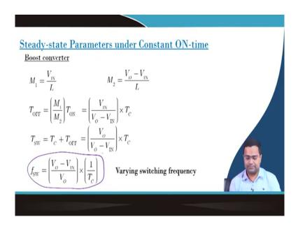
In a boost converter, if we derive this on time slope, off time slope and then if we derive the switching frequency, it is a function of input output voltage and the on time. So, switching frequency varies with the input voltage.
