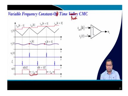
And this should be constant off time. So, it should be constant off time and it should be peak current mode control sorry peak current mode control. Here, it is similar to peak current mode control where the off time is fixed, you can see the off time is fix. And we are taking the sample whenever the switch hit the upper limit; that means, that means in the mono shot timer when sorry it should be taken here.
