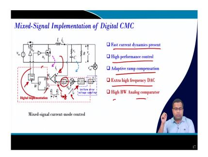
So, one of the solution if you go for mix signal; that means, since our current loop requires faster. It is the fast dynamics and we need to retain the ripple information we should not now digitize the current loop. So, current loop let it be in the analog domain, but the voltage loop is digital domain; what is the advantage, because since you have a compensator in the voltage loop. So, we can play with the tuning that we have learned right.
