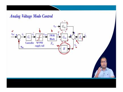
So, in this we will start with analog voltage mode control. We have already discussed in analog voltage mode control. We have a reference voltage and we are trying to design a voltage regulator. This is my actual output voltage, and this is the sensor. Typically, this could be a resistive divider. And then this sense voltage goes to our this is the sense voltage here.
