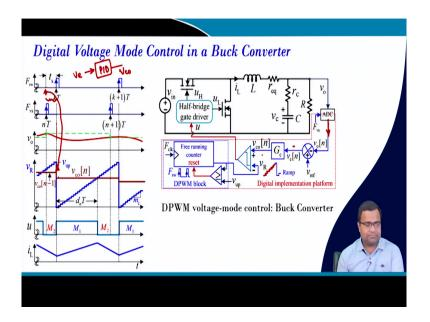
Now, coming back to our digital controller as I said this is A to D converter your sample voltage, this is error voltage, then control voltage and now, this sawtooth waveform is generated inside the digital control. So, there is nothing outside ok. And we have this if we want to draw the waveform and we have to discuss, generally we need to send the sampling command much earlier, because it will take some time to convert the continuous time signal like it a.
