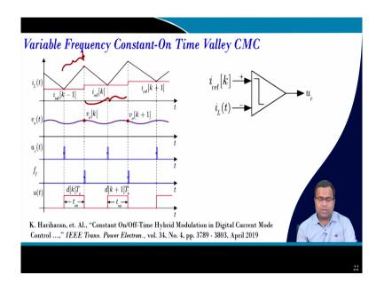
And if you go to variable frequency constant on time control in fact, in the next lecture, we will show the waveform the experimental result that it remains same and if we go to constant on time control, it is also a variable frequency control we have learned. Again, we can use this event-based algorithm.
