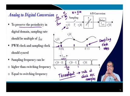
So, we call it as a latency. So, for us this is the one of the most important. This latency will decide what is my delay? So, if we take pipeline ADC. The pipeline ADC is the delay is generally decided by the number of stages pipeline stages. So, if there are 6 numbers of pipeline stages. So, your delay will be 6 times of the sampling clock.
