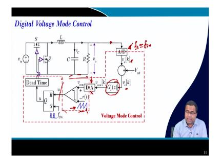
Now, if you go to digital controller. So, we discuss one A to D converter and we discuss this sampling rate to be roughly we are taking same as the switching frequency right. And then, after this sense voltage comes inside, it is the digitized one; that means, it is both sample as well as quantize.
