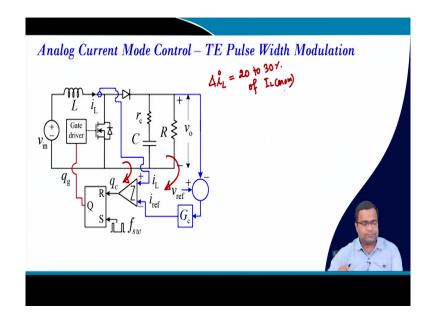
Then, we can do regular PWM operation. If you go to analog current mode control; current mode control, we have 2 loop control. One is the current loop, and the other is the voltage loop right. And we know the current loop voltage loop can be sampled once per cycle, but the current loop cannot be like that, because the current ripples are quite large.
