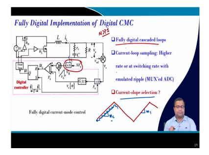
In case of fully digital, we know that the now the current loop is in digital domain, but we need to sample either at a high sampling rate or we can sample. That means a cascaded loop. Either you can use the higher sampling rate; that means, this N; N can be very, very high, but
