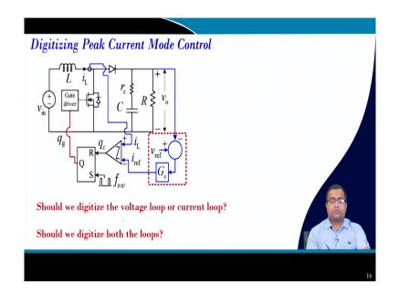
So, the next question how do you digitize the peak current mode control. Should we digitize the voltage loop, should we digitize the current loop, or should we digitize both the loop?
