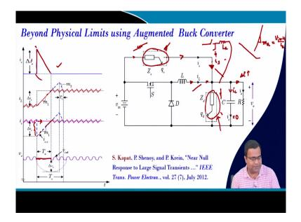
Then we have to go. We need to make some circuit rearrangement, otherwise it is not possible. So, during the load step up transient, we need to provide an extra path because what happens? During the step up process, suppose you know if you take the dash line your
