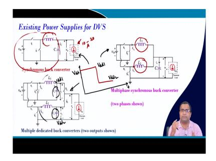
Now, we want to find what are the existing method. So, the simplest example is a synchronous buck converter, simple normal buck converter where it is supplying to a processor right. So, this is a very standard one. If the current requirement of this processor is low, let us say it is like 10 to 20 ampere kind of rating, a simple buck converter should be sufficient.
