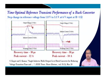
So, the time optimal performance if I show a result that has taken from this and it is given in this paper that if we want to change the voltage from 1.8 to 3.3 volt you can see it takes a longer duration right. So, it is 30, it is taking almost 30 microsecond and with a high peak current, the peak current is very high, this peak current is very high.
