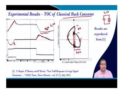
But because this particular phase, it is in DCM mode discontinuous current when the inductor current become 0, when i L is 0. So, as a result your capacitor is simply discharging across the load across the load during this you know when i L equal to 0. And since the load current is low, the rate of discharge is very slow and it is taking lot of time ok and there is a huge overshoot.
