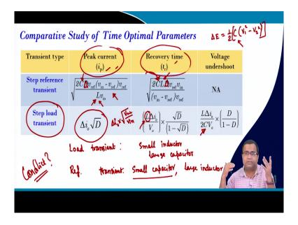
And if you compare the time optimal parameter, if you take the load step transient, we saw the peak current is basically delta i 0 D where it was like a delta i 0 into reference; that means, ref by V in right and you saw at higher input voltage it was low, but lower volt voltage it was very high.
