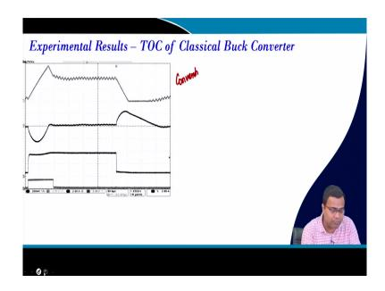
So, one of the way we told that we use a resistive network ok. And this is the time for optimal recovery of a conventional buck converter. So, this is like a conventional buck converter or I will say a classical buck converter, which is given where we are using a diode. So, we are using a diode base converter.
