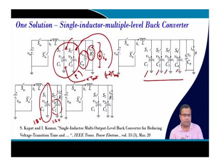
So, one solution how to cut down because we found the problem load transient and reference transient has some conflict in the design. So, one of the solution we take you know one inductor and two pre charge capacitor two pre charge capacitors. And at any point, suppose you want to change from one voltage to the other voltage. Suppose you use this capacitor as your output can and let us say this is sitting at 1.8 volt and let us say this is pre charged to 1.2 volt.
