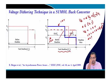
So, we can use a voltage dithering technique; that means, if my required voltage in the deadline is my dotted line right then I can use a higher voltage to finish early, but that I said that it is not a good way. So, you will lose more power than I can take two different voltages. Suppose I have two voltages are available. So, one voltage is my v 2 as I said maybe at 1.8 volt and other voltage is my v 1.
