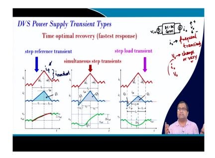
But before I move forward, we need to first understand what are the different type of transient in dynamic voltage scaling because you know as usual when a DC-DC converter is supplied a DC-DC converter a supply to a processor load; that means, here a processor load we have a supply here V in.
