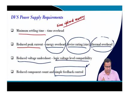
So, the DVS power supply requirement we need a minimum settling time or basically minimum recovery time and that is why we talk about time optimal control, time optimal recovery that will reduce because the linear control cannot meet that, right? Then, we also want to reduce the peak current because if the peak current during the transient if you go back to this, so, to the peak current, generally we determine this current, this is my peak current right.
