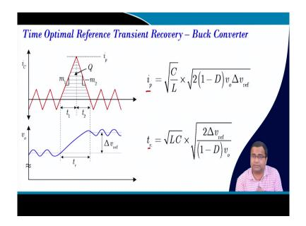
Now the time for optimal reference transient recovery. So, we talk about load transient recovery, now we are talking about reference transient recovery in reference transient you have a peak current and here the voltage has to change from v v ref to v ref plus delta v ref and we have discussed the peak current recovery time these two are the parameter that we are going to discuss.
