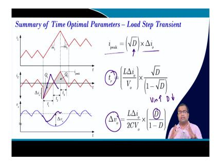
So, they we generally consider a bank of capacitor. So, summary of time optimal load transient; we know the peak current, recovery time and the load step undershoot. And this undershoot can also be reduced again if you if duty ratio decreases; that means, if input voltage decreases, then naturally this undershoot, because if you can increase this. You can see during this time the voltage will only fall and then rise, so; that means, undershoot will also reduce ok.
