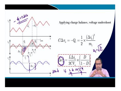
Another part. If we apply charge balance to the output, we want to compute this output voltage undershoot. So, it is nothing, but if you take this charge, because during this time the voltage will fall right. So, if you take this particular scenario. So, our Q 1 is nothing but C into delta V 0 right. If you do that Q 1. So, yeah it should be minus of Q 1, because we are considering delta V 0 magnitude; that means, it is the magnitude rather than the sign.
