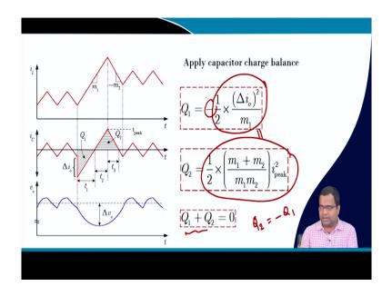
So, next applying charge balance we have Q 1. We have Q 2 and what is my charge balance. The sum of the two charges must be 0 capacitor charge balance and then it will balance.
