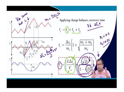
So, apply charge balance. What is the recovery time. We know t 1 we have already computed t 2 plus t 3 if you substitute. And I have already told what is m 1 plus m 2. So, it will be L delta i 0 that is my load step size into V 0 and square root of D divided by 1 minus duty ratio D; that means, this recovery time I can show you.
