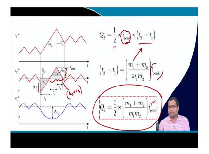
Next, what is my Q 2? Again, the height is i peak half into height i peak into this duration is my t 2 plus t 3 t 2 plus t 3 right. So, this is here and what is t 2 by t 3 that we know m 1 plus m 2 divide by m 1 into i peak. And if you substitute here, and what you will get; Q t equal to
