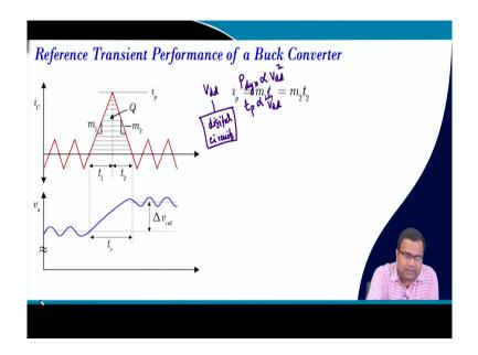
Now, for a reference transient, because if we consider this DC-DC converter is supplying a digital processor load; that means, V d d of a digital circuit. So, this digital I can say digital circuits. So, there are millions of maybe transistor digital transistor and each of them requires a V dd. So, this overall V dd will be supplied by DC DC. Now, we know that the dynamic power the dynamic power of any cmos processor is the square of V dd.
