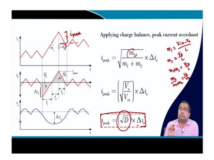
Now, what is my m 1 and m 2 for a buck converter? so; We got this relation. For a buck converter, m 1 is V in minus V 0 by L. And what is my m 2; m 2 is V 0 by L, because we are taking minus of m 2 say m 2 is V 0 by L. Then, what is my m 1 plus m 2 it will be simply V in by 1 and. So, if you take m 2; that means, my m 2 by m 1 plus m 2 is nothing, but V 0 by V in and this is exactly is coming square root of V 0 by V in.
