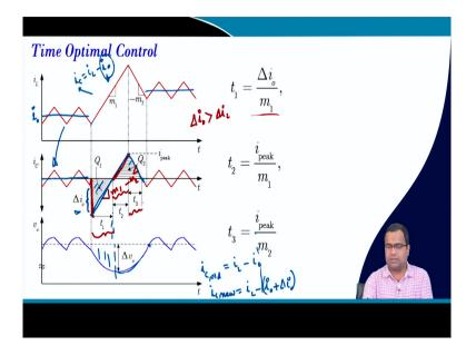
So, the time optimal recovery will start with this using capacitor charge (Refer Time: 4:14) which is a very standard method. So, you see, the capacitor current is nothing but for a buck converter in continuous conduction, because we are talking about a synchronous buck. Here, the average inductor current is the average load current right, and that is before transient and after transient, it is delta i 0 plus delta i 0.
