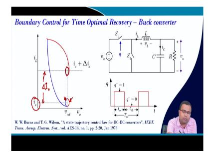
And this trajectory looks something like this; that means we have initial load current of i 0 here, our initial load current i 0 here and then, there is a load step transient with a step size of delta i 0 and then it will reach to another trajectory. Here again, the blue one is the on-state trajectory and the red one is the off state trajectory and it will reach to the next operating point in one switching action ok.
