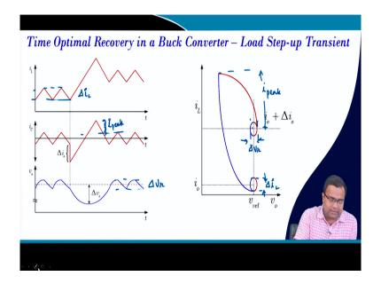
Now, the timing diagram looks something similar; that means, earlier we talked about the phase plane trajectory, where this ripples if you see if you consider the ripple here; that means, if you consider the ripple parameters here, this is our inductor current ripple and which is same as our inductor current ripple. And this is our output voltage ripple delta V r and which is nothing but our this parameter or this parameter delta V r ripple parameter.
