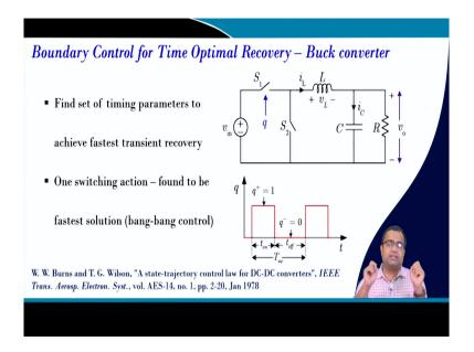
So, first we want to recapitulate the boundary control for time optimal recovery. And that we have already discussed in the previous lecture that we need to set find a set of timing parameter to achieve the fastest response. And that actually turns out to be a one switching action. So, we need to formulate all the parameters in order to ensure that our transient recovery happens in one switching action, then we can ensure the fastest transient or the optimal time optimal recovery.
