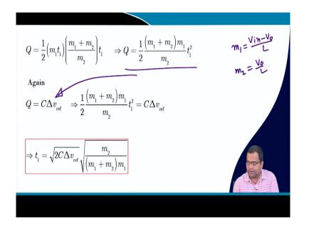
Now, the Q is this we can write by simplification. And we know that Q equal to C into delta V ref that we have told, because whatever charge you are injecting, it will ultimately raise the voltage level. And if we equate these two here, if you substitute here, then we will get this expression. So, your t 1 can be found from this relation and we know m 1 equal to V in minus V 0 by 1 and m 2 equal to V 0 by 1 for a buck converter.
