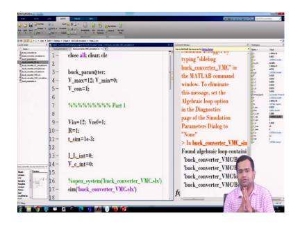
Now, the output voltage has gone high, it is too high because you are using 50 percent duty ratio, but V con what should be the V con? The control voltage you know in order to achieve the duty ratio so, let us say if we set 12 volt here, 12 volt and 1 volt so, you can set V con to be 1 volt, then duty ratio will be accordingly generated.
