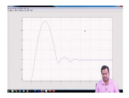
And you can also see during transient, the startup logic is something which is unacceptable, the output voltage reaches 3 volt which is not at all acceptable.
