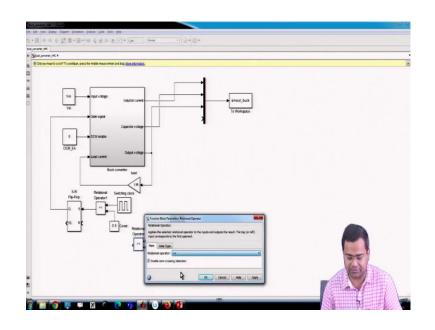
And here, I can use just 1 percent because it is just the edge, we require the clock; clock edge ok fine, this is my DCM, that is my constant that means, this is something like constant and now, I have to use a relational operator and here, it is used to reset that means, we have to reverse the logic. As long as V con is above, it should be high so, it should, we should now reverse the logic because in order to operate this.
