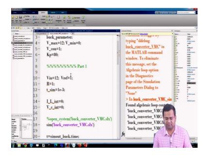
So, that means, we created a transient case study in the part 2, we have changed the load resistance and so, if we want to increase the proportional controller gain let us say 80, how does it look like?
