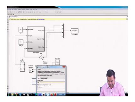
And this R-F flip flop because we want to implement our trailing edge modulation technique. What is the set pulse for this flip-flop? The set pulse for this flip-flop again, flip-flop cannot take, there can be double if you try to run it because this is the double data, data type is a double, but it require a Boolean function so, we need to set another
