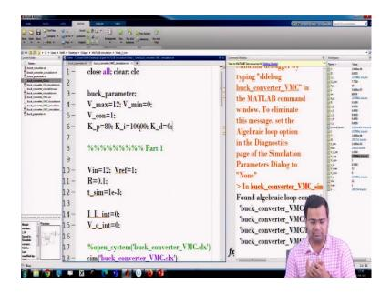
The controller again you can plug in here and you can accordingly create K p equal to this, then K i equal to maybe 10000 and initial we are taking K d equal to 0. Now, I can run it.
